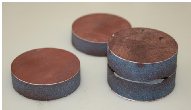
Fig. 3. Cylindrical laboratory samples of the ceramic filter elements used for hematite concentrate dewatering.
