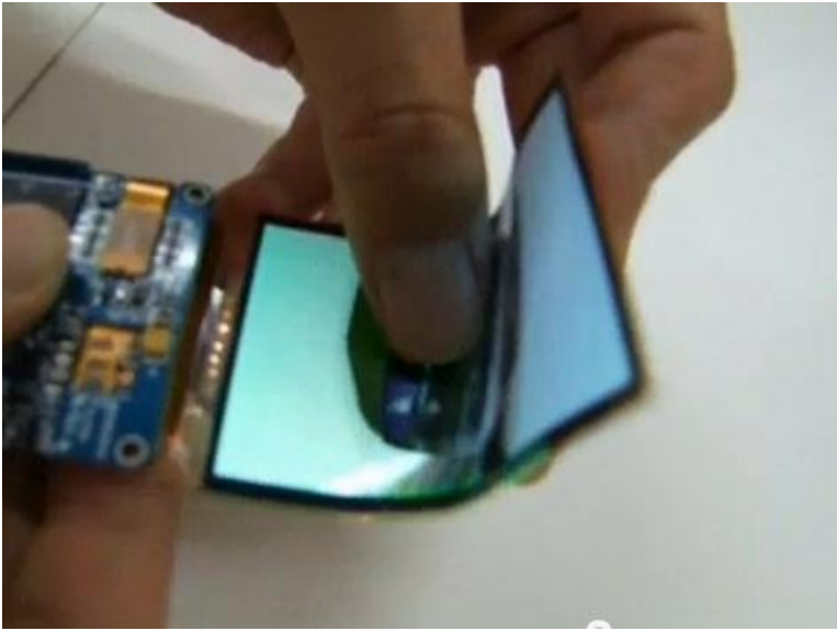
Figure 25. Samsung's prototype mobile phone with a very flexible display. (Technology-Update.us 2010)
