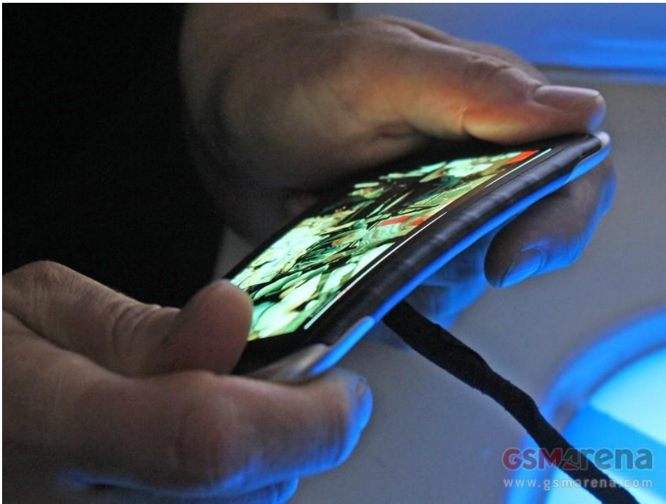
Figure 24. A Nokia prototype mobile phone that uses its bendability to operate the phone. (Arena 2011)
