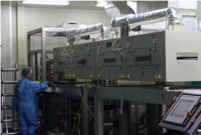
Figure 34. Printer dryers one and two, with the in-feed mechanism below.
