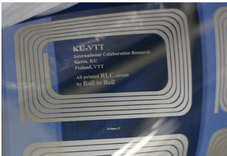
Figure 2. A printed antenna manufactured by the KU-VTT Joint Research Center in Seoul Korea.
