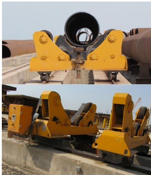
Figure 1 Rotational mechanism for stationary pipe welding [23]
