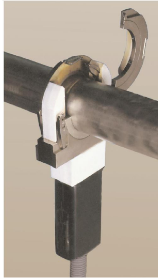
Figure 4 Standard enclosed orbital weld heads can be used to weld tube size from 1.6 mm up to 152.4 mm and wall thicknesses up to 4 mm [4]
