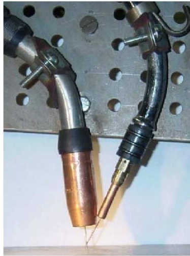
Figure 29 Welding gun arrangement of consumable DE-GMAW process [144, 156]
