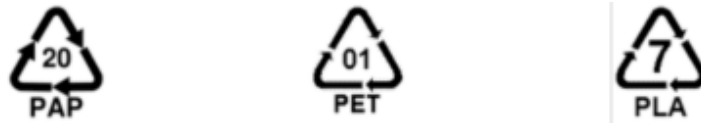
Figure 13. From left to right: recycling symbols to corrugated board, PET and bioplastics. (Recycling codes 2013)
