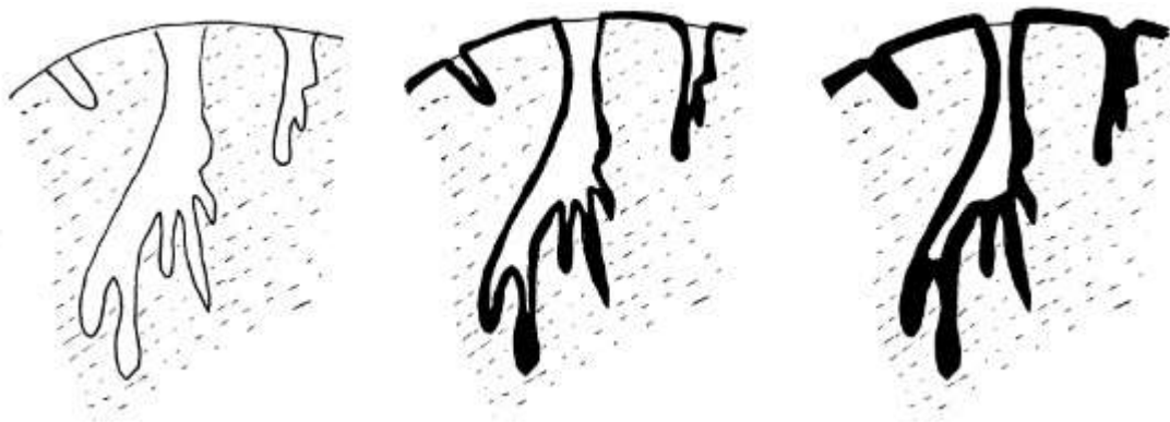
Figure 8. Pore plugging on calcite during gypsum formation
