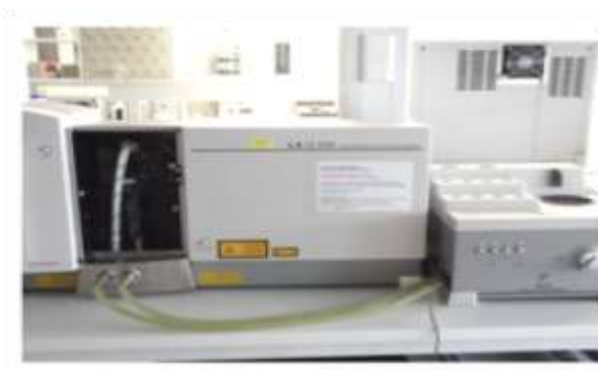
Figure 4. Laser diffractometer LS13320 Beckman Coulter (USA)
