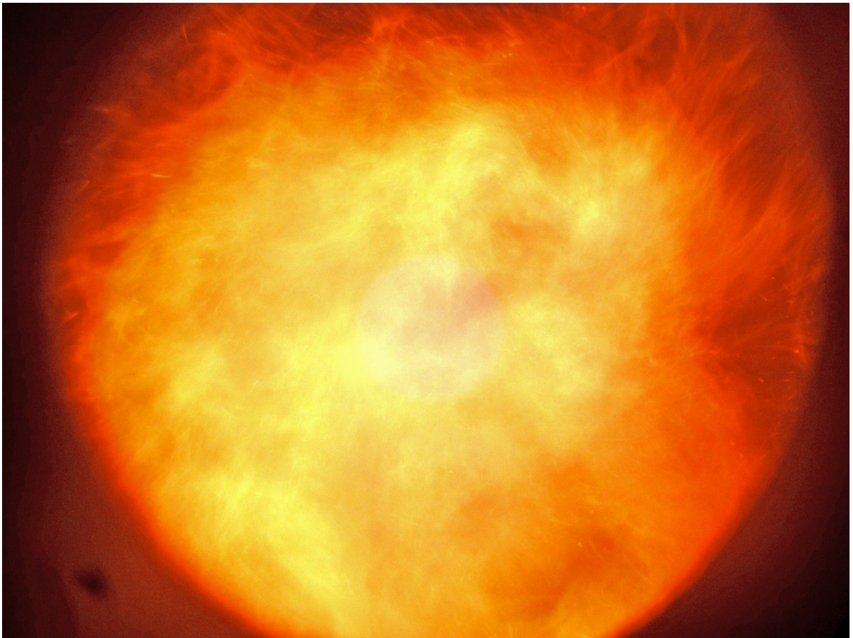
Figure 3. Pyrolysis oil flame.
