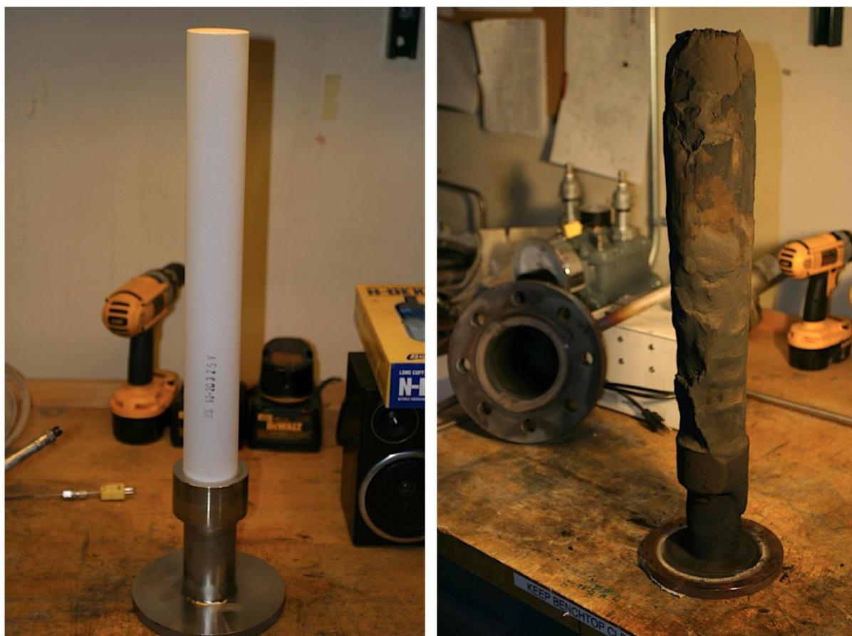
Figure 11. Hot vapor filter candles before and after experiment of 1700 regeneration cycles. (Brandvold 2011)
