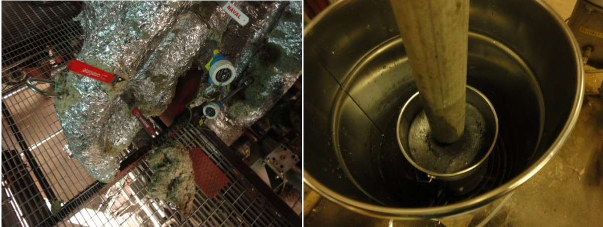
Figure 20. On the left: The valves for taking the sample. On the right: the sample in the bucket.
