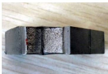
a) Crystalline, shinning brittle fracture, absorbing little energy on impact.
