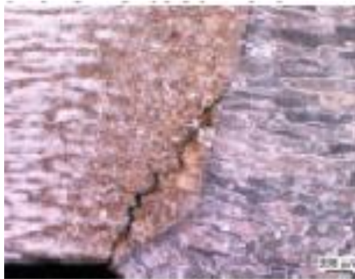
Figure 41 HAZ crack caused by insufficient preheat [86].
