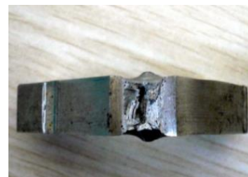
b) Fibrous, dull ductile fracture, absorbing relatively large amount of energy on impact.
