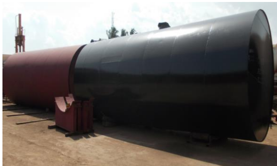
Figure 12. Manufactured tank for underground storage of fuel.
