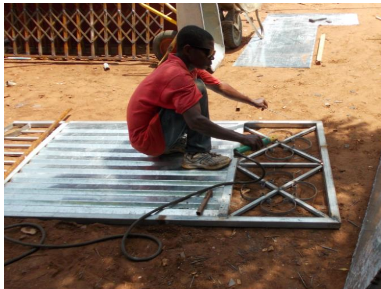
Figure 11. Squatting position during a welding operation on the floor.
