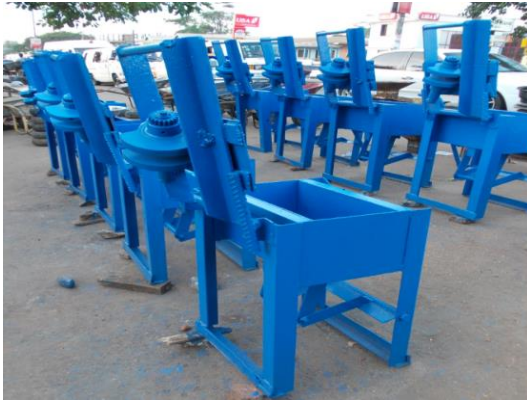
(a) Cement Block Making Machine
