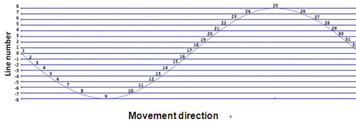
FIG. 3. The places of adjustment points of scanner power along the sinusoidal wave.
