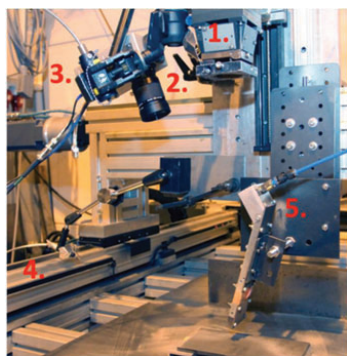
Figure 2. Experimental setup. 1. Precitec welding head. 2. High-speed camera. 3. Illumination system. 4. Spectrometer 5. Powder feeding nozzle.
