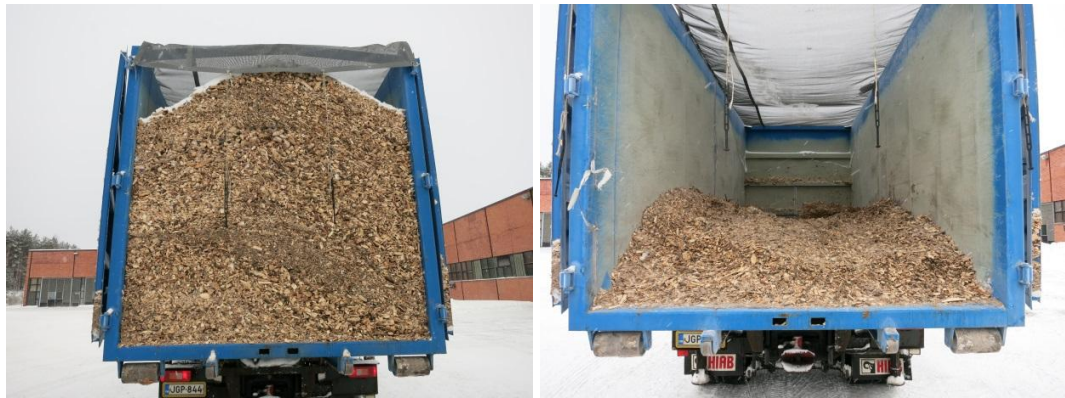
Figure 15 The metal container before the unloading on the left and after on the right.
