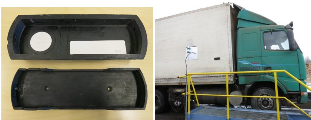
Figure 15 The RFID identifier box on the left and the truck vehicle on the weighbridge of the power plant on the right.
