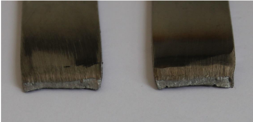
Figure 37. Fracture surfaces of a welded sheet metal test piece.
