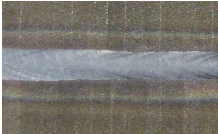
Figure 35. A typical weld surface in one of the SLM test pieces.
