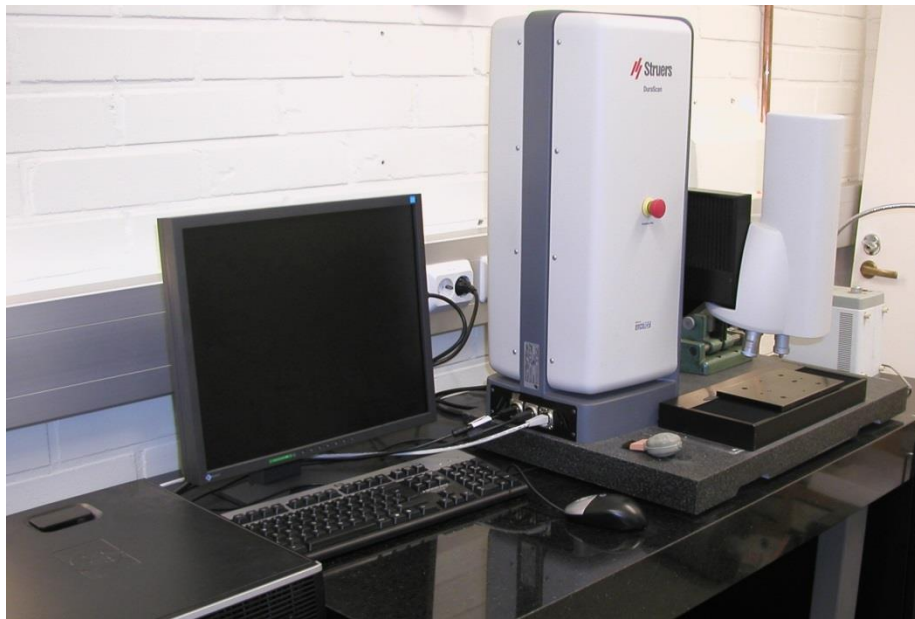
Figure 31. Struers DuraScan-70 automatic hardness testing device used in the study.
