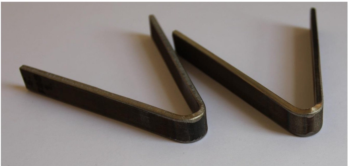
Figure 39. SLM face and root bend test piece after testing with no visible defects or cracks.
