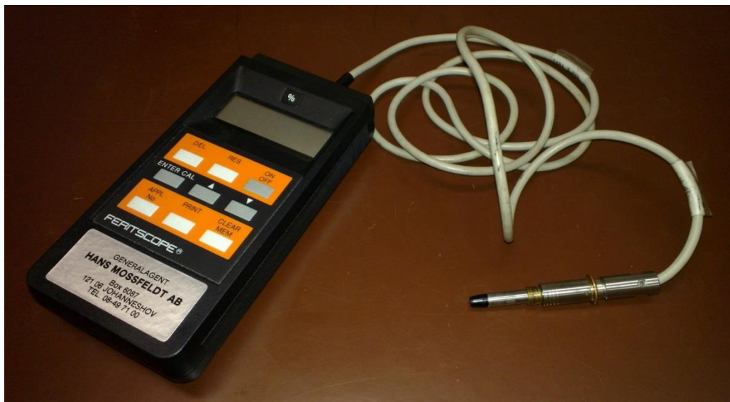
Figure 33. Feritscope MP3 ferrite content measurement device.
