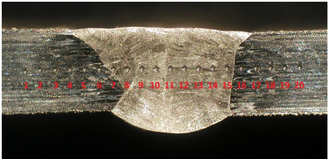
Figure 41. Hardness test measurement points in the weld area of the test piece made with selective laser melting.
