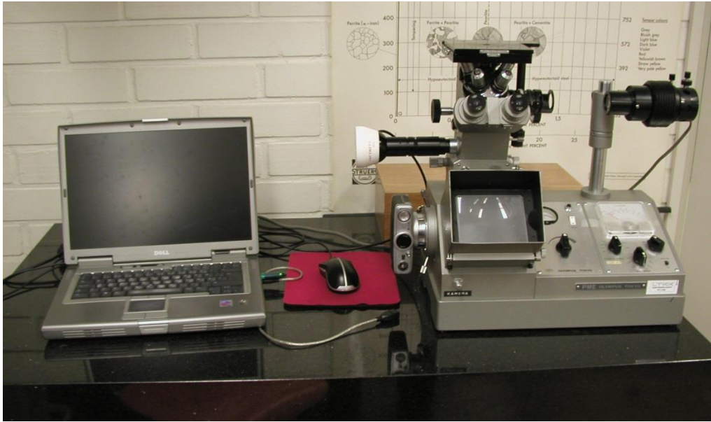
Figure 32. Olympus PME metallurgical microscope equipment used in the study.
