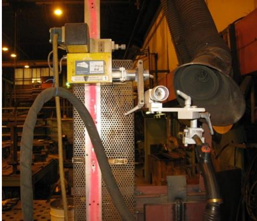
Figure 19. Esab welding carriage on rail with mounted welding gun
