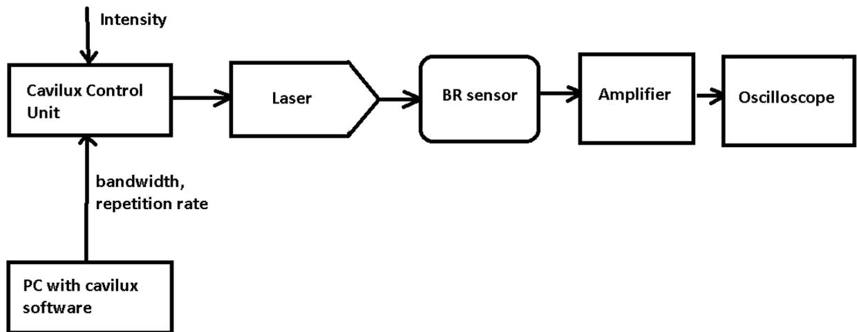
Figure 11. The BR measurement system.
