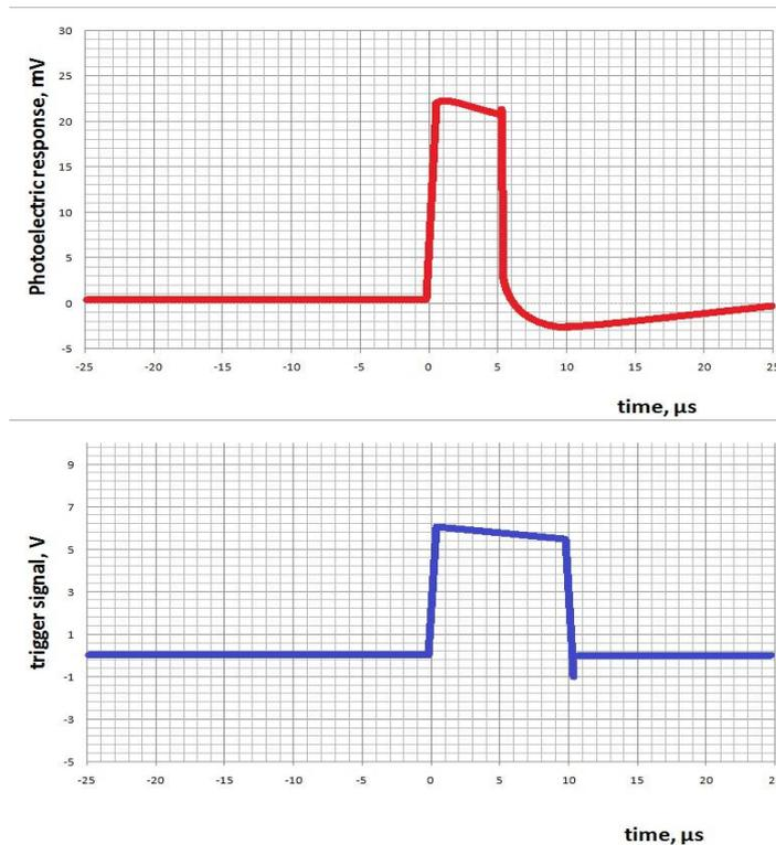
Figure13. The photoelectric response obtained from the BR sensor. The blue line represents the trigger signal (the laser signal). The length of the laser pulse is 10  $\mu\text{s}$ . The shortest pulselength, which gives the signal distinguishable from noise is 50 ns. The repetition rate was 23 Hz.
