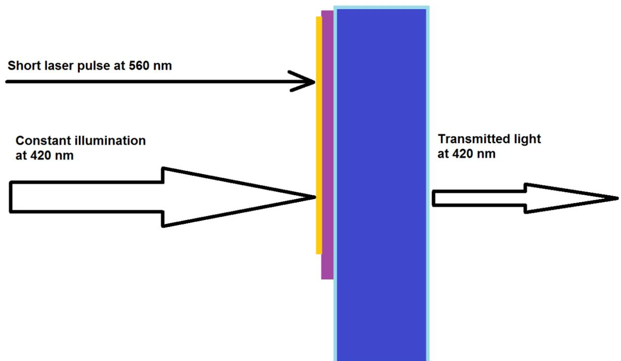
Figure 8. BR absorption measurement setup.
