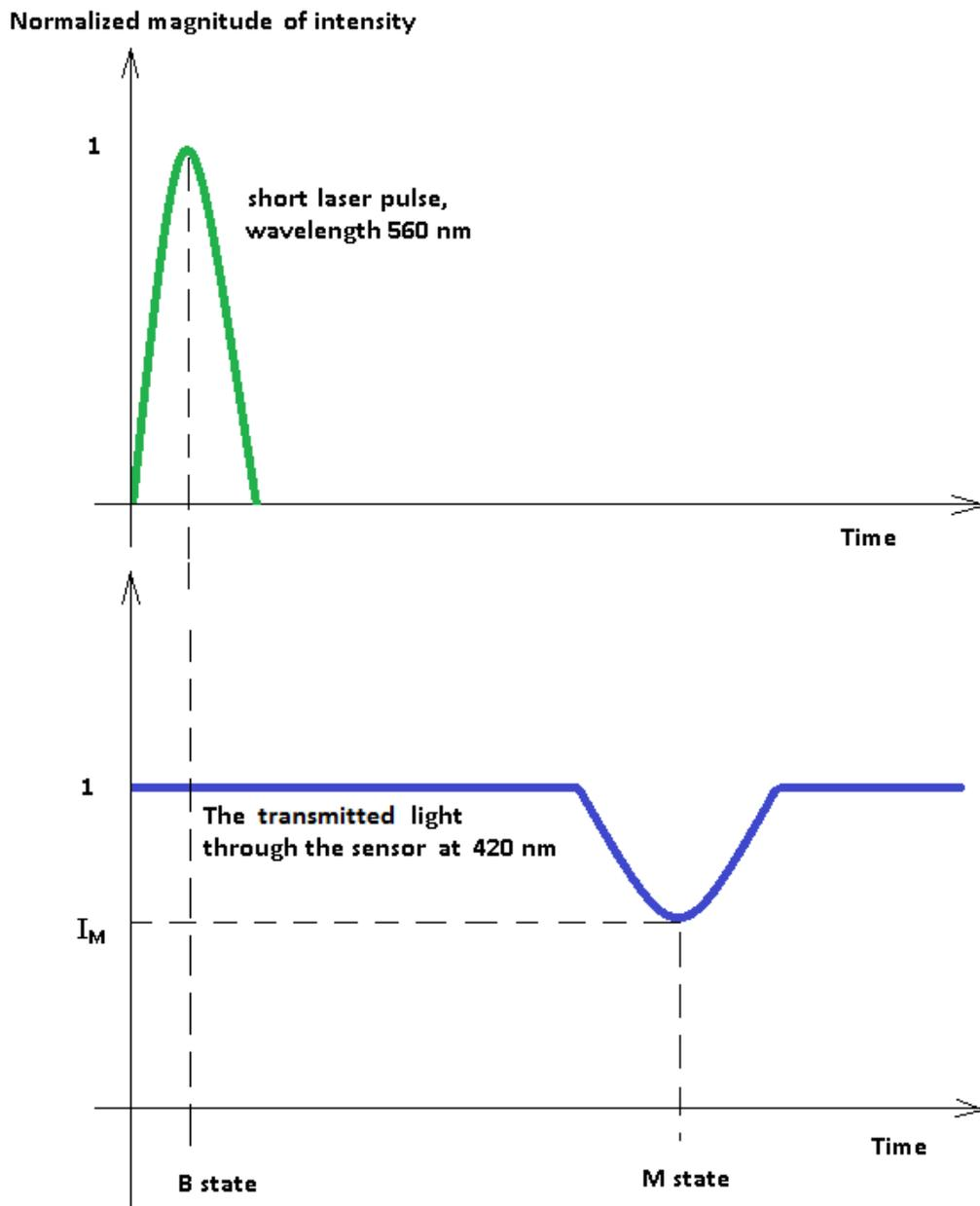
Figure 9. Schematic diagram of the transmitted light intensity. In the M state, the intensity of light is lower at 420 nm.
