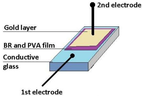
Figure 6. The structure of simple bacteriorhodopsin sensor.
