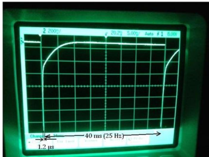
Figure 22. The laser beam signal obtained with the pulse picker device. Repetition rate frequency is 80.04MHz. Pulse width was 0.4 ps on the pulse picker device. The signal was measured by using a photomultiplier tube.
