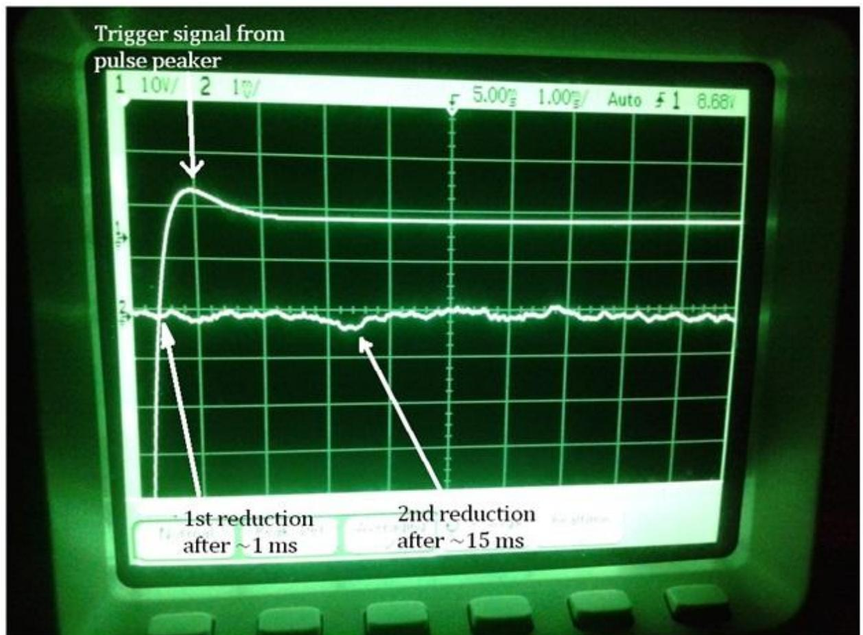
Figure 23. The liquid sample transsion at 420 nm measured with a photomultiplier tube in according with the scheme presented in Figure 21. The signal is obtained by averaging 16000 samples to reduce the noise.
