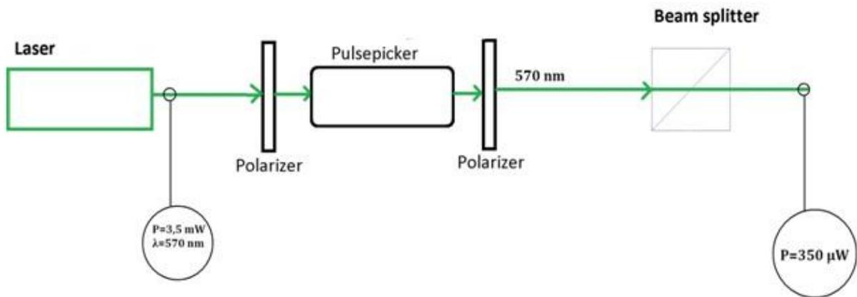
Figure 15. Estimation the average power of the laser signal setup.
