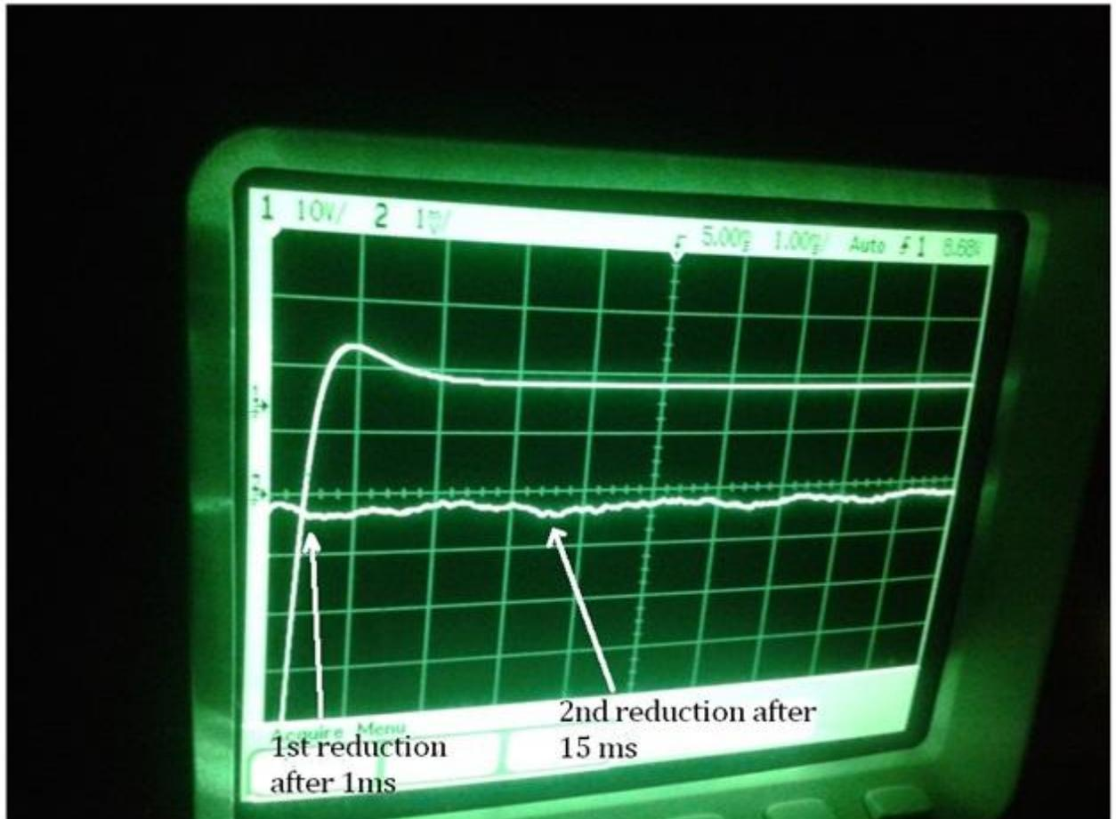
Figure 24. The dry sample transmission at 420 nm measured with a photomultiplier tube with the setup presented in Figure 21. The signal is obtained by averaging 16000 samples to reduce the noise.
