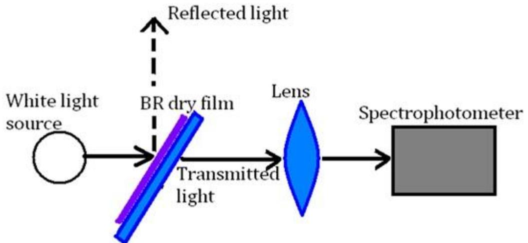
Figure 16. Transmitted spectrum measuring setup.
