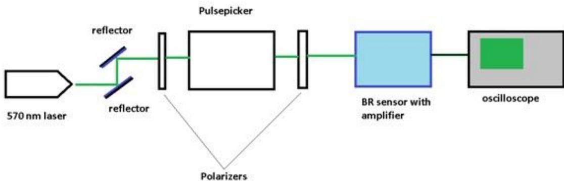
Figure 19. Photoelectric response measurement setup.
