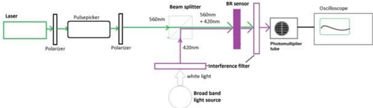
Figure 21. The measuring setup for optical response measurements.
