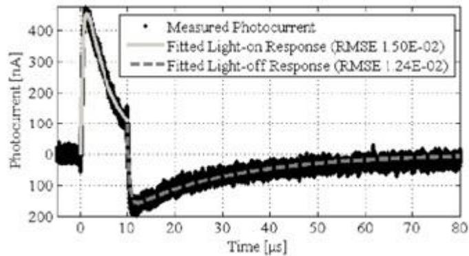
Figure 14. The photoelectric response from [16] – the same experiment with old amplifier.
