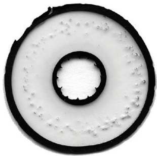
Figure 1.5. Cable wafer with extensive voids [17].
