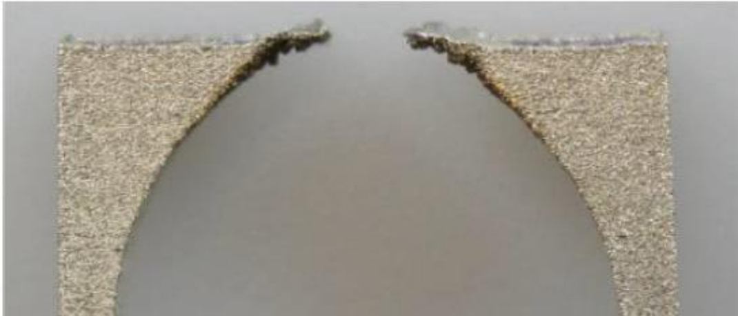
Figure 13. Result of uncontrollable curling (modified from: Guido et al., 2015, p. 667).
