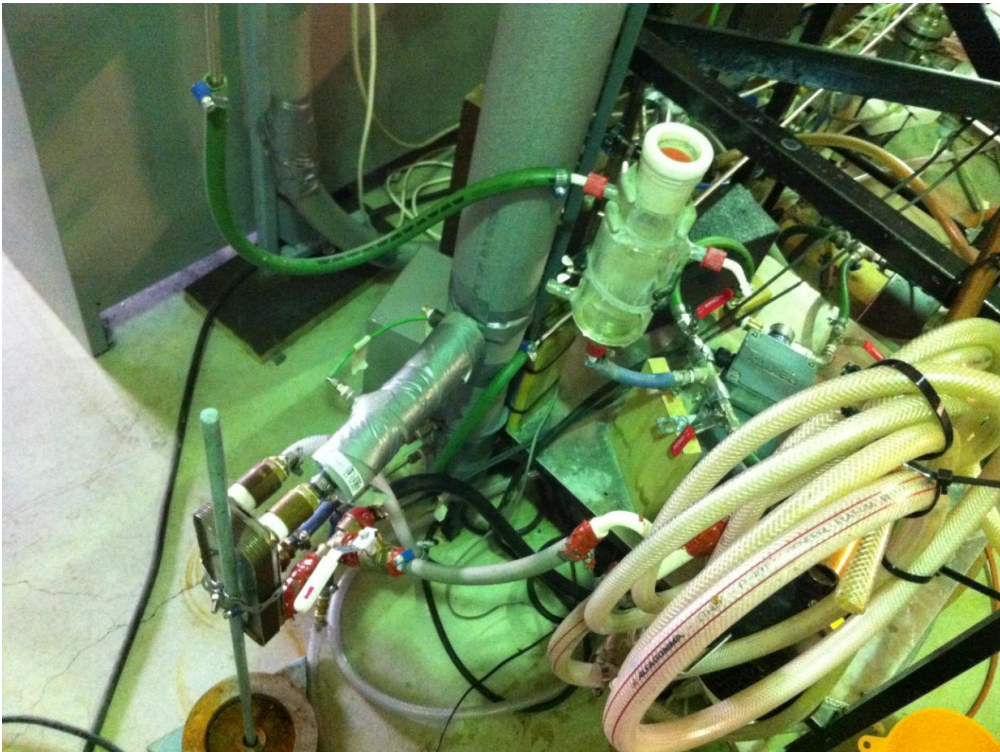
Figure 11. Experimental Setup (Heat Exchanger and nanofluids reservoir)
