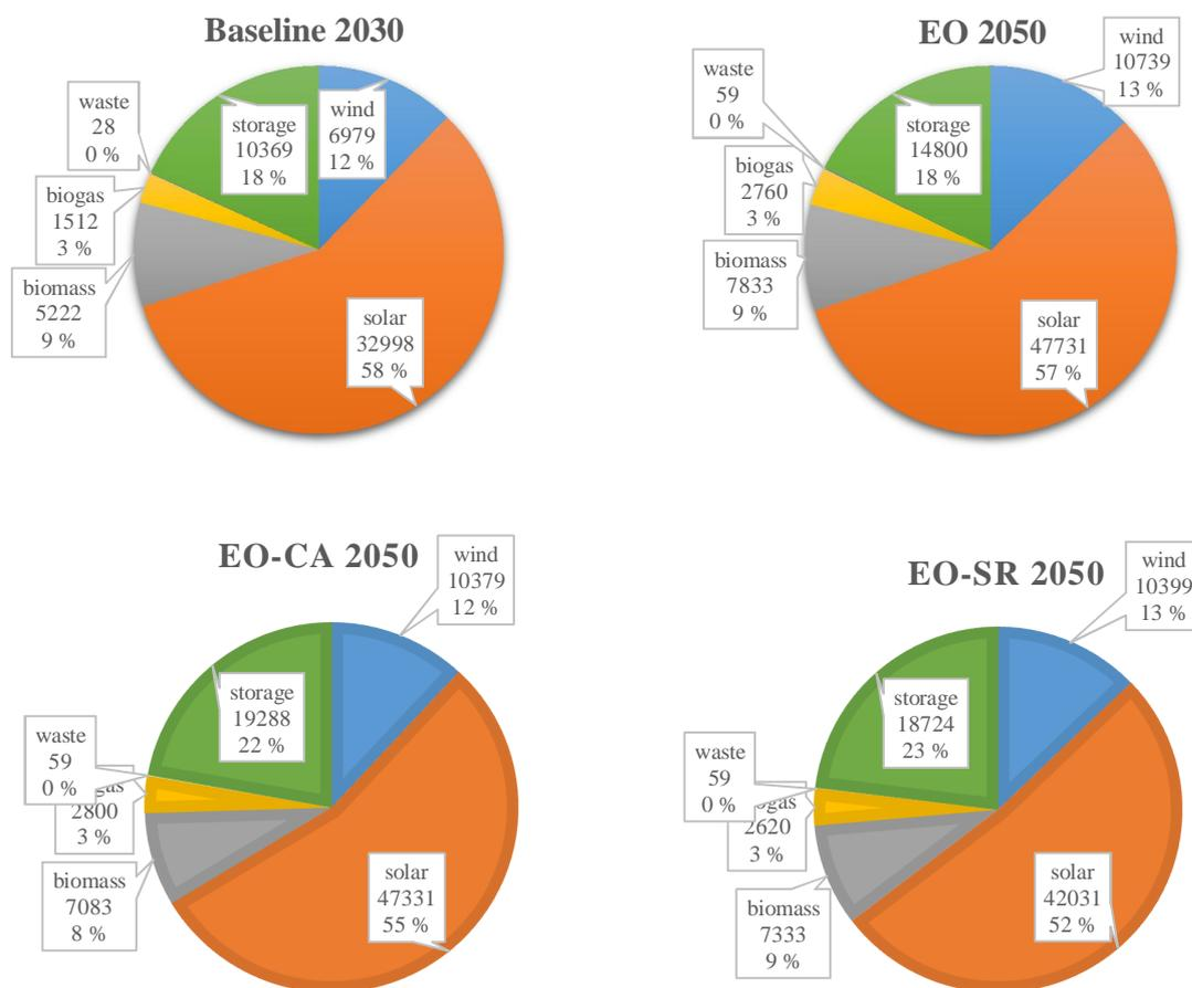
Fig. 8. Installed capacity (MW, in percent of total) by technologies under three different market designs (year 2050)
