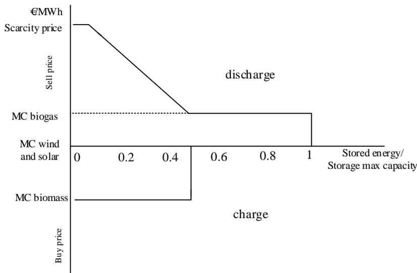
Fig. 2 Bid curve of a battery storage
