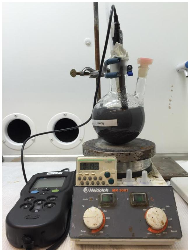
Figure 13. Experimental set up for nitrate reduction reaction.
