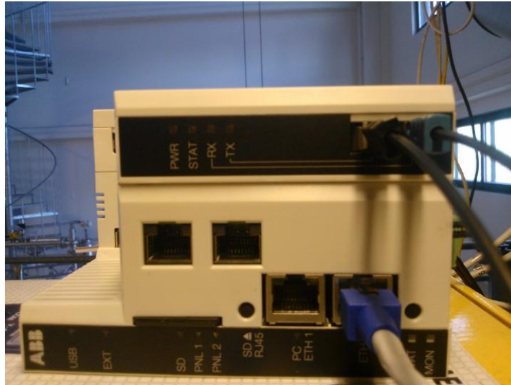
Figure 5.3 ABB NETA-21 remote monitoring tool with additional NEXA-21 module. To access device data loggers, DDCS communication with the frequency drive was implemented by connecting NEXA-21 to the VSD with fiber optic cables. NETA-21 is connected to the laboratory network with Ethernet cable to gain access to the web UI and data logger settings.
