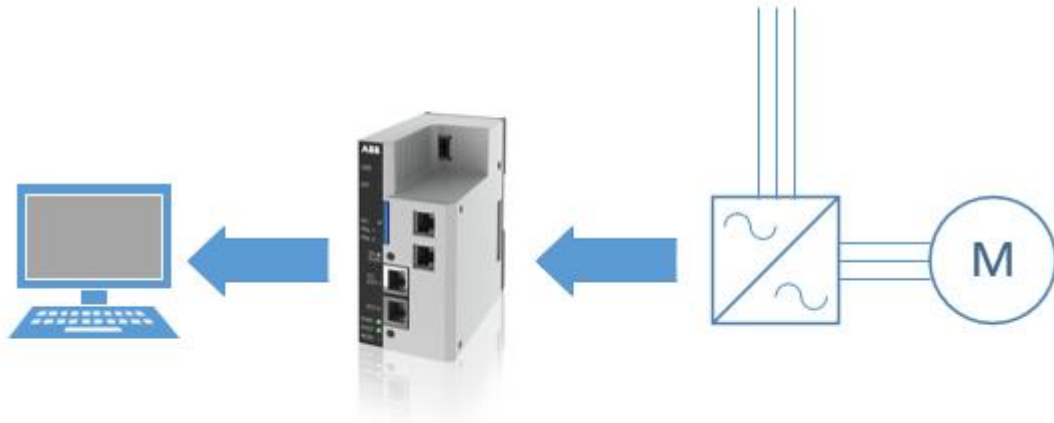
Figure 4.1 Simplified data flow diagram. The VSD is controlling the motor while NETA-21 monitors and logs the desired variables from the VSD. The data logged by NETA-21 unit is stored and later accessed with a PC for further analysis.
