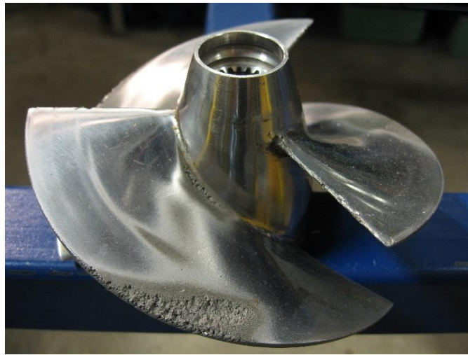
Figure 2.4 Cavitation damage on propeller. The vane edges are damaged due shock waves caused by imploding bubbles (Wikipedia, 2006).
