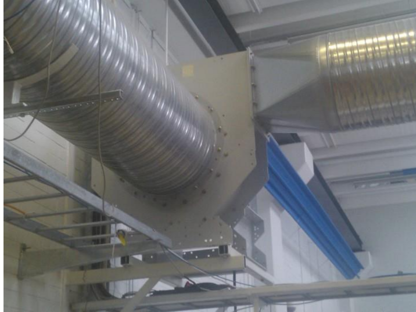
Figure 6.1 FläktWoods Centripal EU 4 MD 630 radial blower in a test setup. Flow measurement is done from the suction side and the operation point is controlled with a damper at the discharge side of the system.
