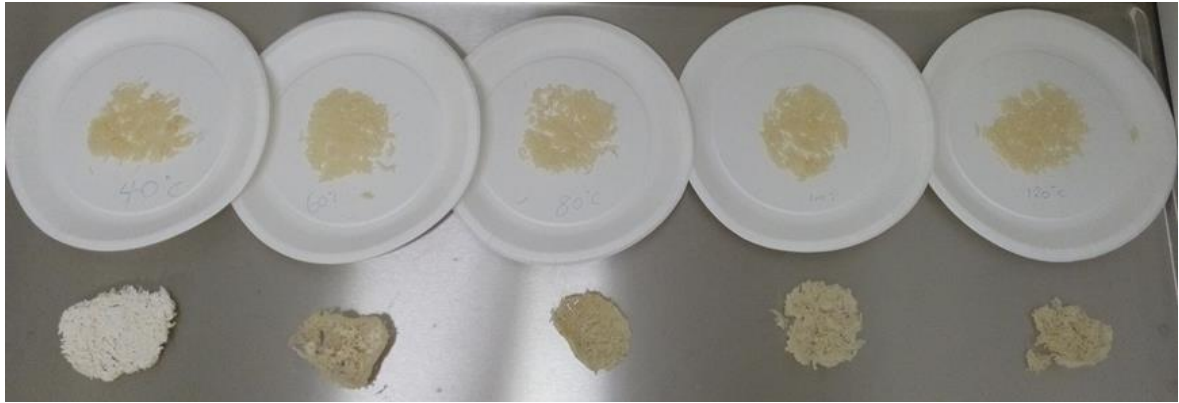
Figure 55. The results of drying tests – (Up row) are the atmospheric dried samples, (Down row) are the vacuum dried ones. The temperatures are written on the plates from the left to right: 40°C, 60°C, 80°C, 100°C, and 120°C. The sample at 40°C in vacuum drying is different from the rest and has a bigger volume but the same weight, because of the low temperature this sample almost freeze-dried.
