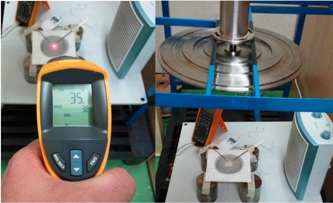
Figure 56. (left) Temperature measurement method using three thermometers, (right) drying set up at Pusonics.
