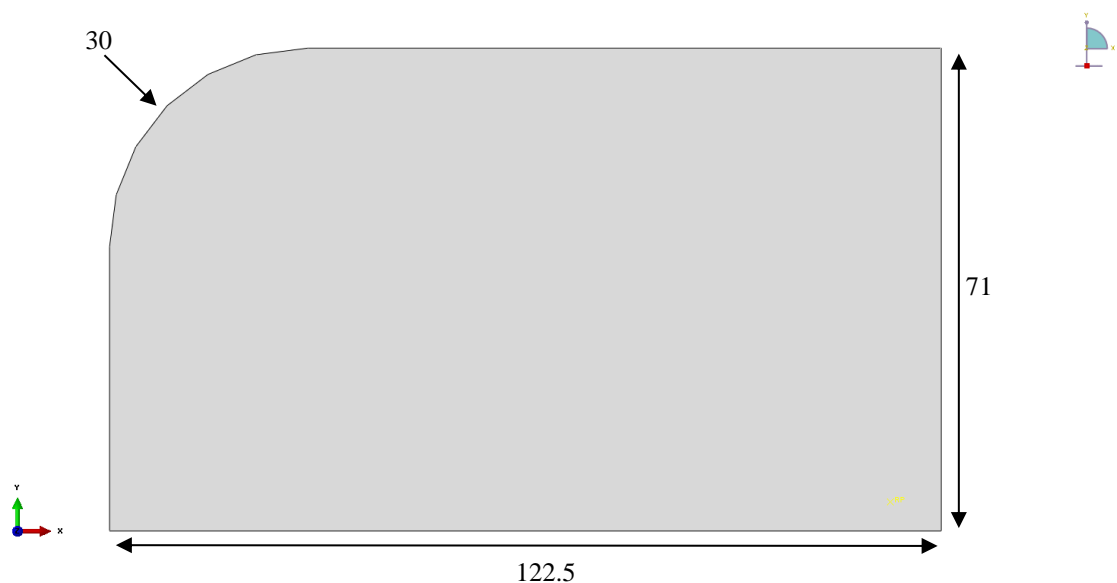
Figure 12. Top view of male die.
