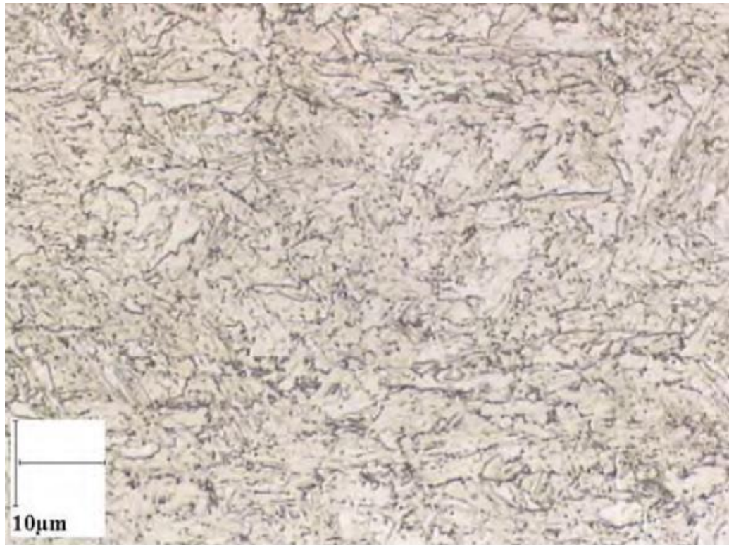
Figure 5. Microstructure of hot rolled CP steel (Keeler & Kimchi 2014, p. 2-8).
