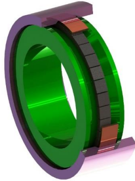
Fig. 4.2. 3D model of the actuator that works on the voice coil principle.
