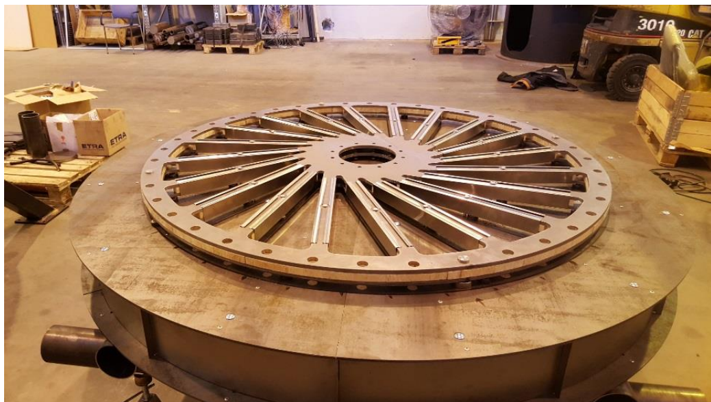
Figure 37. Assembled wheel face on top of torsion box.
