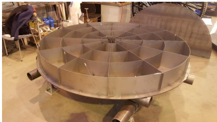
Figure 31. Installed 1 mm thick circular and radial walls.
