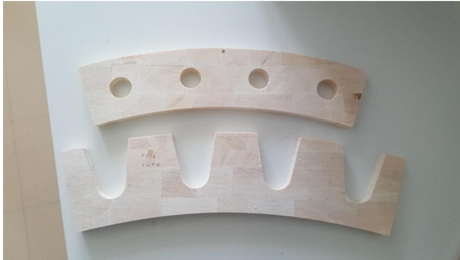
Figure 27. CNC cut balsa spacers for rotor and stator rims.
