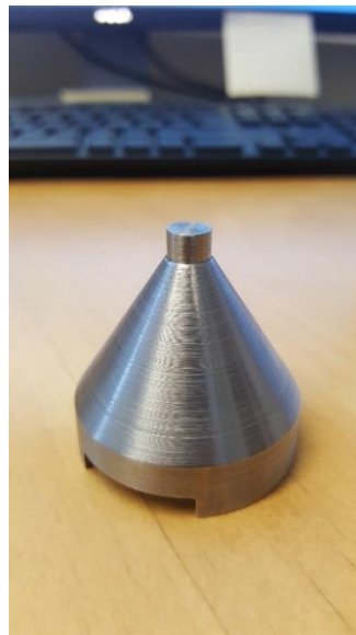
Figure 34. Prototype of spacer tool for wheel face assembly.
