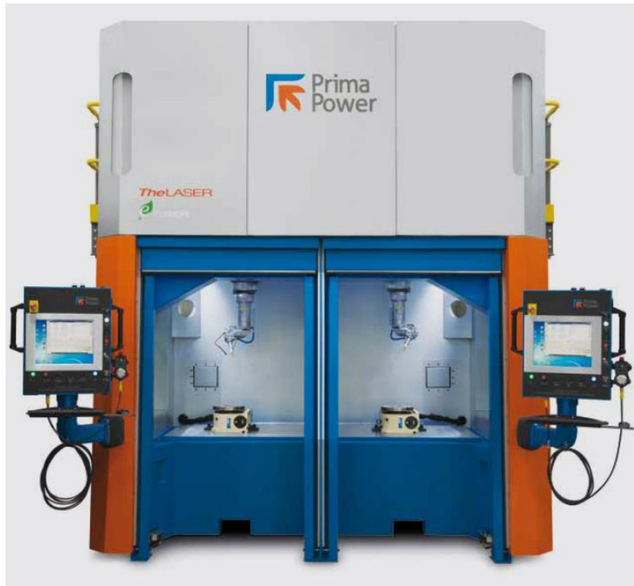
Figure 14. Prima Power Laserdyne 606 D 3D dual laser processing machine (Prima Power 2017, p. 22).
