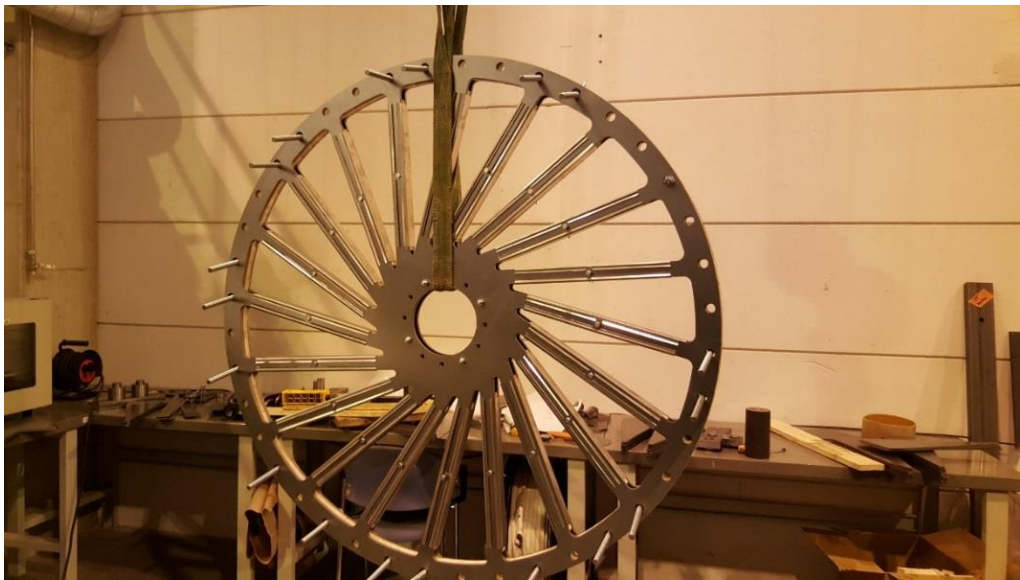
Figure 29. Assembled prototype of rotor wheel face of 750 kW machine.
