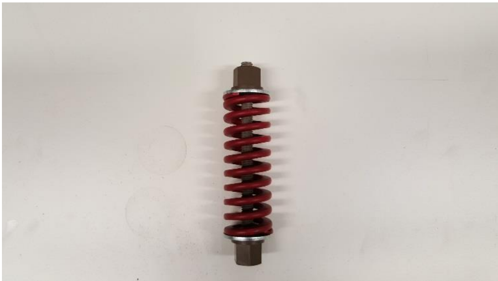
Figure 16. Test assembly for fiberglass vinyl ester stud bolt.
