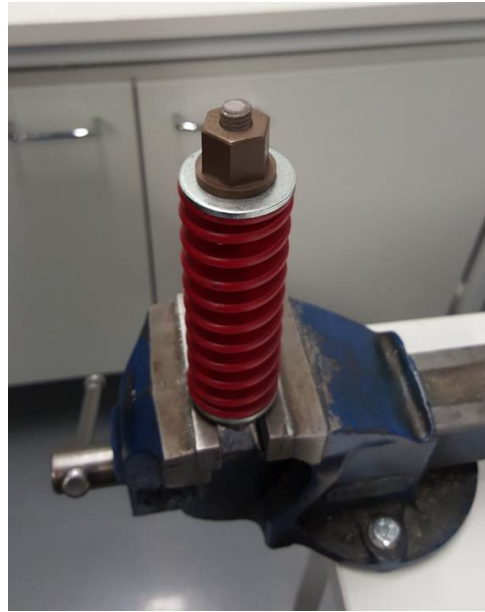
Figure 17. Bolt test assembly attached to a vise.
