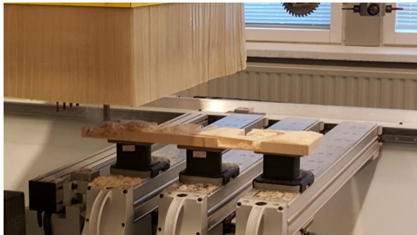
Figure 26. Cutting process of balsa wood part.
