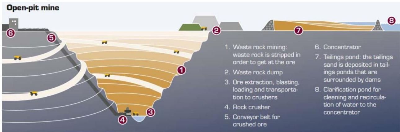
Figure 6. Layout of an open-pit mine (Boliden, 2016).
