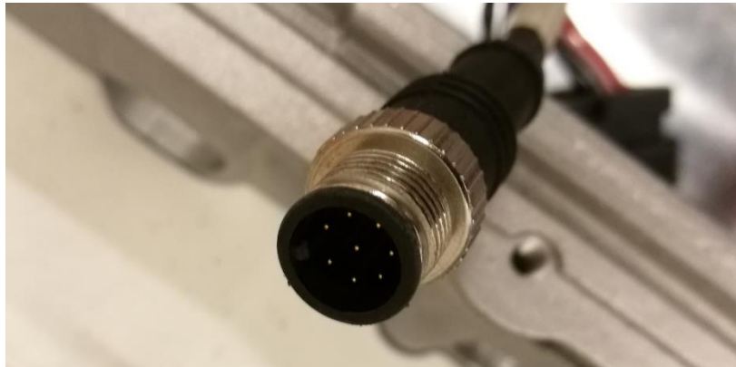
Figure 2.13 The RS-485 connector used in maintenance connector interface. It is used to connect a PowerMASTER inverter to a computer with serial connection. There is a small overhang inside the connector and a metal spiral on top of the connector.
