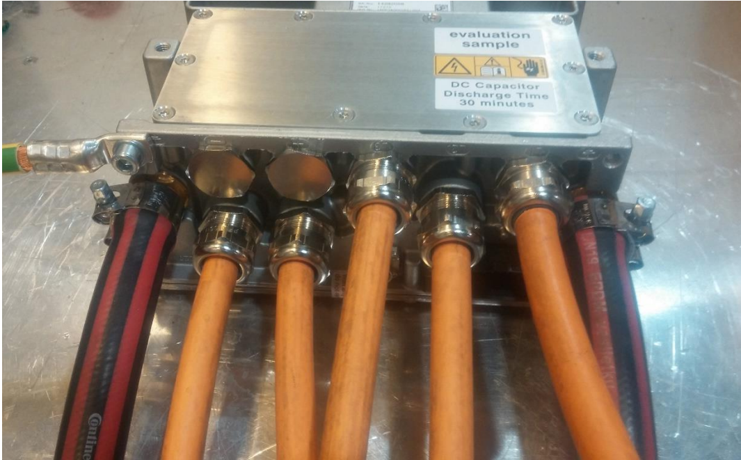
Figure 2.11 PowerMASTER with connection box lid installed. Use 10 Torx screws to install the lid and use 4 Nm tightening torque.
