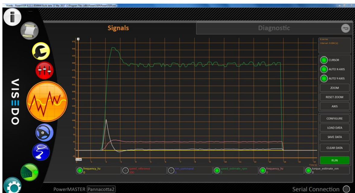
Figure 3.7 Signal logger in PowerUSER application. Logger can be started by clicking run on the right bottom corner and stopped by clicking the same button. Logged data is from a motor start and a stop with 300 RPM reference speed.
