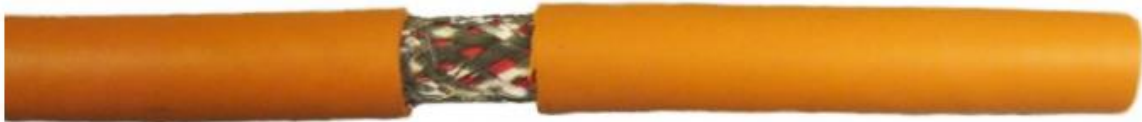
Figure 2.5 High-voltage cable with braid screen visible. Do not completely remove the cable sheath before the cable gland is installed (Visedo 2016a).
