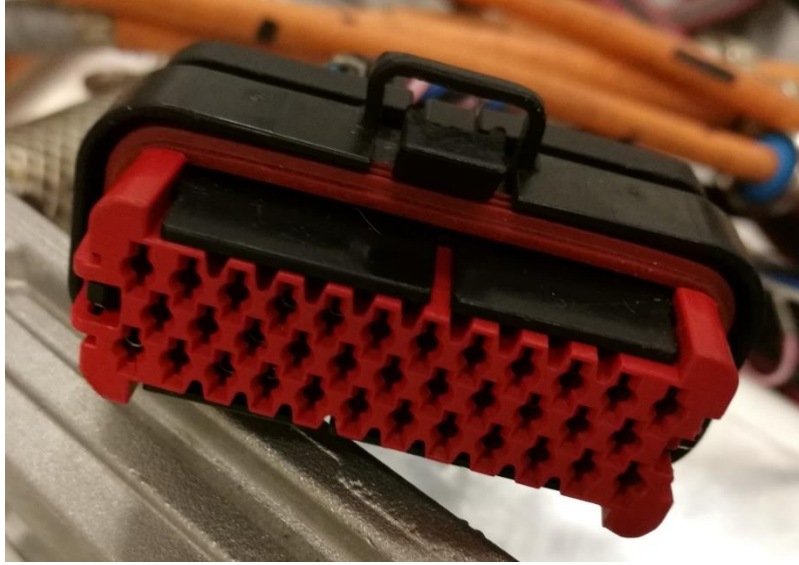
Figure 2.12 The 35-pin X1 connector used in connecting PowerMASTER inverter for low voltage signal connection. The plastic locking system is on the top of the connector.
