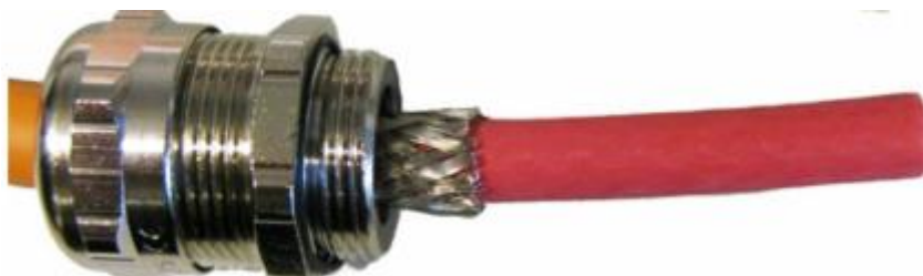
Figure 2.6 High-voltage cable with cable gland installed. Push the cable gland against the sheath of the cable and cut the braid screen 10mm from the bottom of the cable gland (Visedo 2016a).
