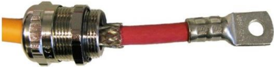
Figure 2.7 High-voltage cable with the cable lug installed. Cut a piece of the inner cable sheath from the end of the cable with same length as the body of the cable lug, insert the lug and crimp it in two different places (Visedo 2016a).
