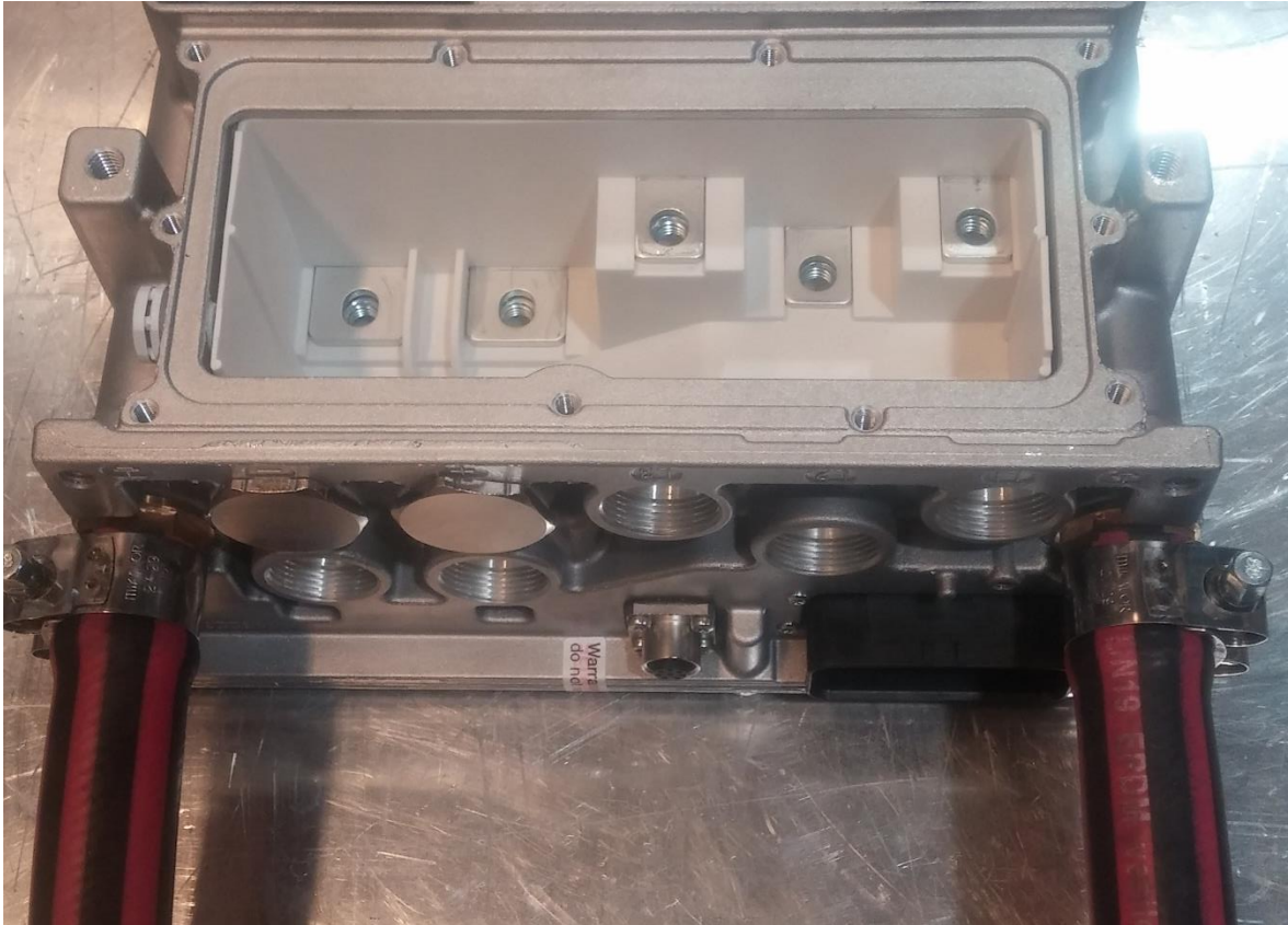
Figure 2.1 Liquid cooling installed on PowerMASTER inverter. Use hose clamps or clips to compress the joints.
