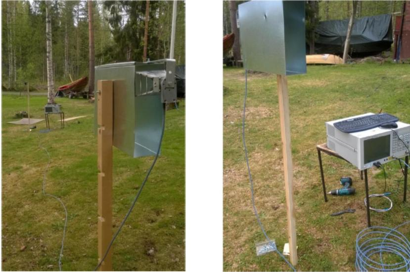
Figure 4.4: Testing microwave attenuation behaviour through spraying port models at the yard. The antenna is in back position in the left figure.
