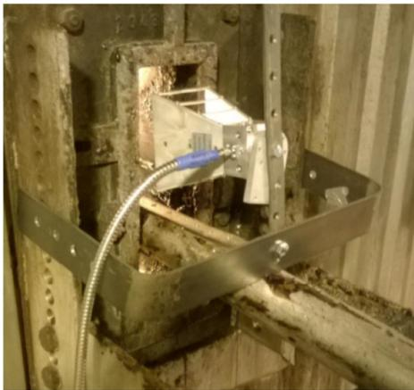
Figure 4.1: Horn antenna LB-20180 at sprayer port of a kraft recovery boiler for attenuation and noise measurements.
