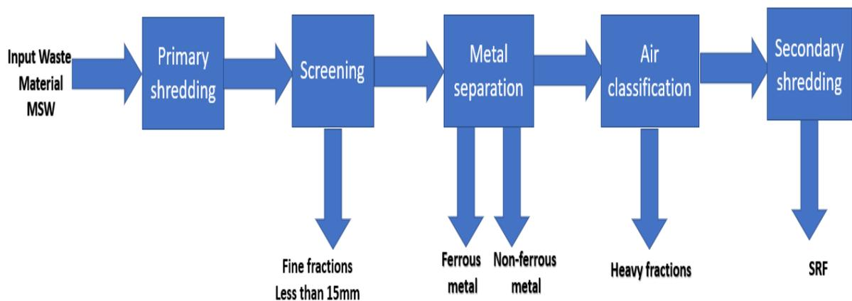
Figure 18: The mechanical treatment of mass solid waste (modified from Nasrullah et al., 2015).
