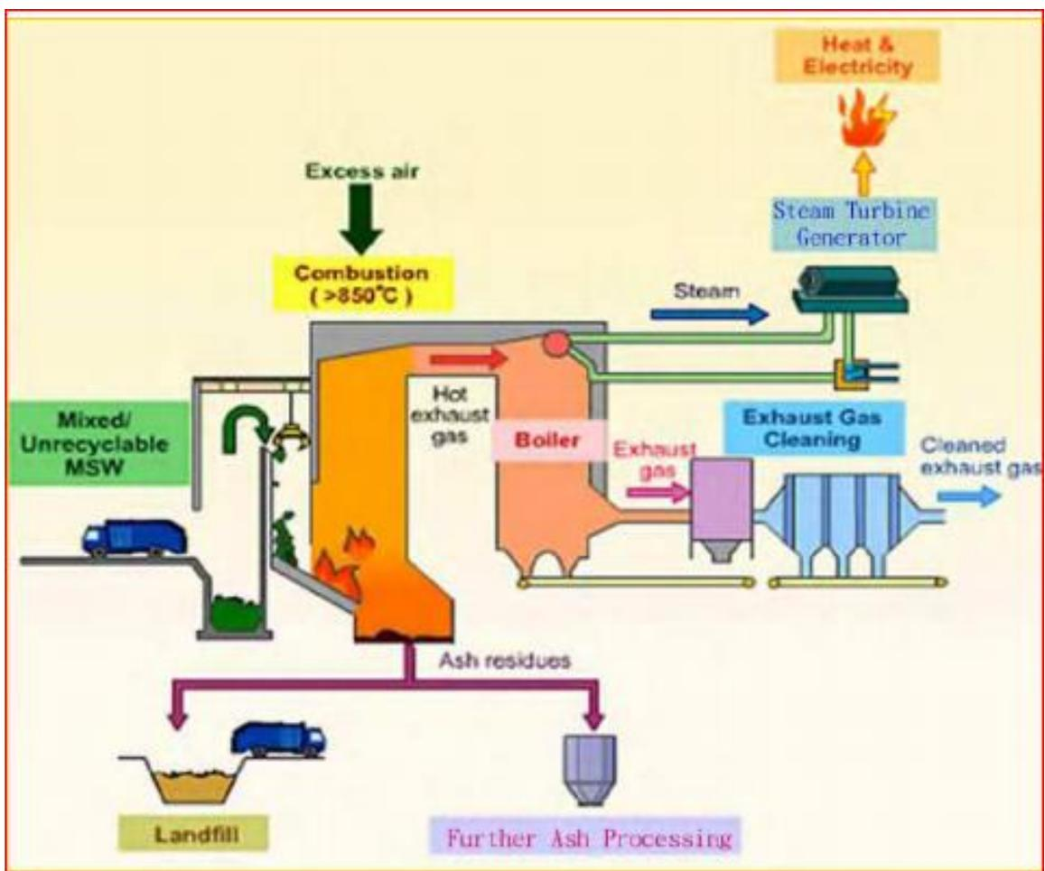
Figure 7: Incineration process (Moustakas and Loizidou, 2010).
