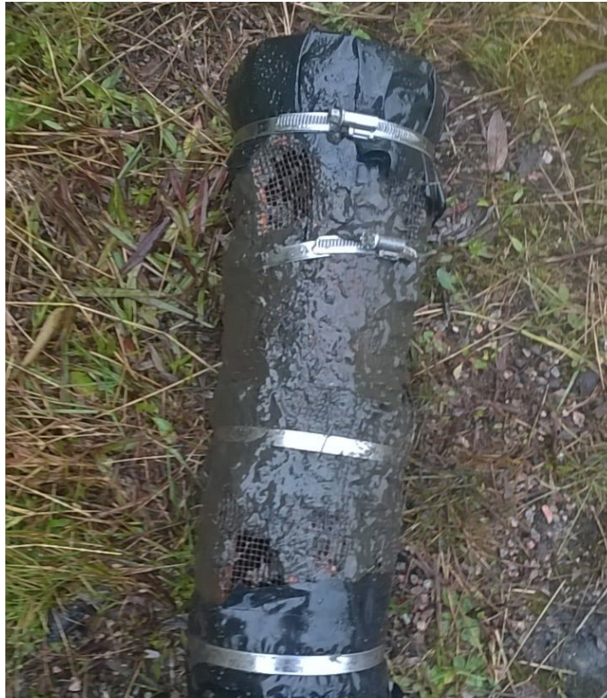
Figure 36. After some weeks use, solids in reject water have blocked the sieve.
