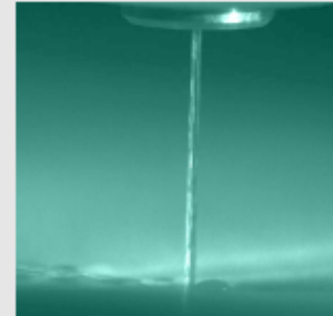
Water jet for cutting of paper, jet thickness 200 microns. Measurement of width & size.
