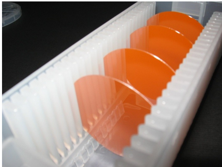
Figure 2. GaP Wafers grown by Czochralski extrusion taken from [17].
