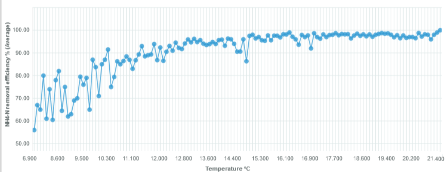
What is the trend of NH4-N removal efficiency % (x) over Temperature °C
