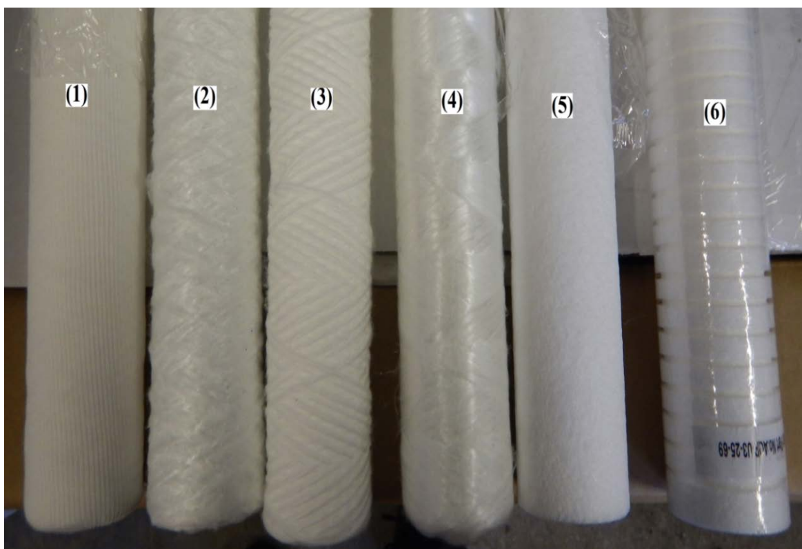
Figure 14. Different types of cartridges used in chemical processes. Cartridges number 1,2 and 4 are made from glass fibre and numbers 3, 5 and 6 from PP. The cartridges from 1–4 are wound type filters and last two are bonded type. Thick fabric sock is added around cartridge 1 to prohibit fibre materials detaching to process stream. Cartridge 6 has grooves cut to increase the surface area and reduce clogging. Cartridges have 25 \mu\text{m} retention diameters, except number 4 has 5 \mu\text{m} retention diameters.
