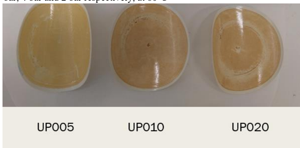
Figure 33: Pictures of UP005, UP010 and UP020 membranes after spent DES filtration
