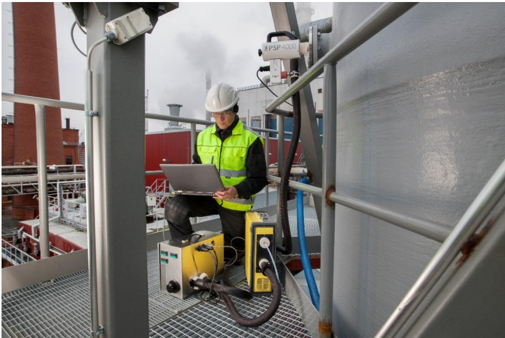
Figure 24 Above pictures A and B show how a measurer works with the FTIR for some industrial flue gas (pictures from Gasmot Oy)
