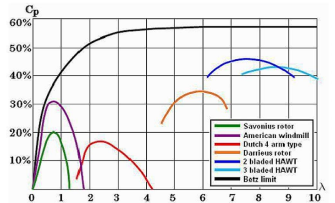
Fig. 3. Power coefficient ( C_p ) versus Tip speed ratio ( \lambda ) of various Wind Turbines [17].
