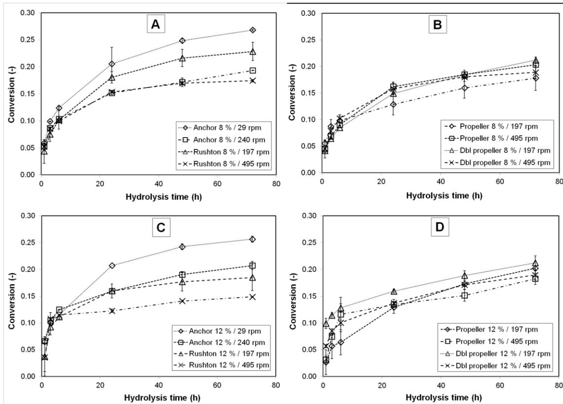
Fig. 3. Effect of rotation speed of the impeller and solids content of the slurry on the enzymatic conversion. Solids content of 8 % (A, B) and 12 % (C, D).
