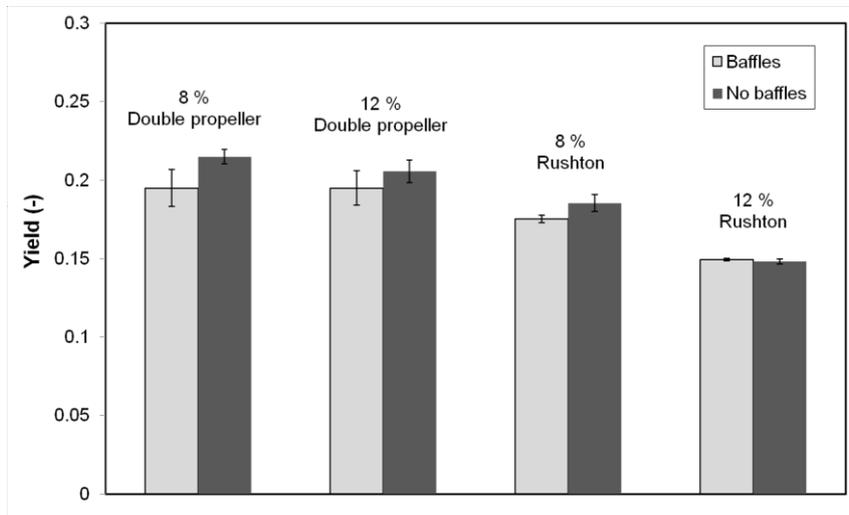
Fig. 4. Glucose yields obtained at different slurry solids content (8 and 12 %) by double propeller and Rushton turbine with and without baffles. The rotation speed was constant, 495 rpm.
