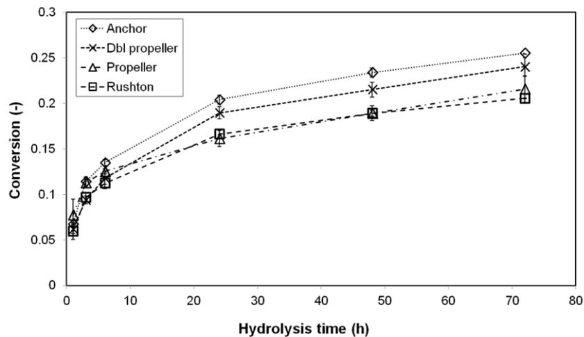
Fig. 2. Performance of the investigated impellers in enzymatic hydrolysis of the model biomass at 10 % solids content, medium rotation speed.
