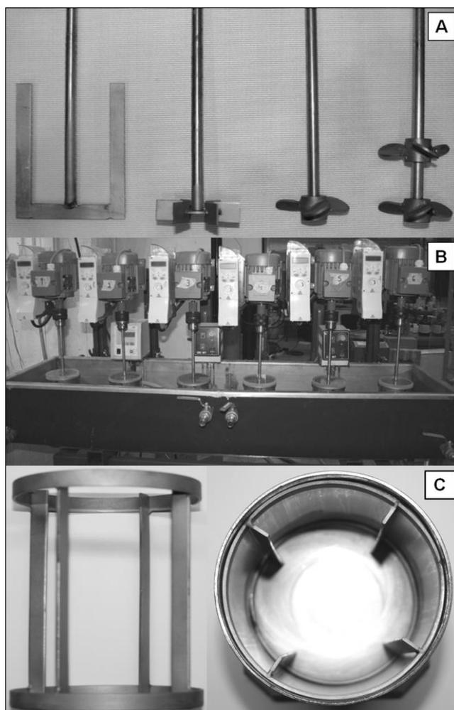
Fig. 1. The impellers left to right (A): Anchor, Rushton turbine, propeller, double propeller. The mixing device (B). The baffles and a mixing tank with the baffles (C).
