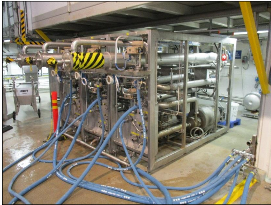
Figure 17 Pilot unit used in experiments. Feed, retentate and permeate lines connected to separate tanks and pumps outside the picture.
