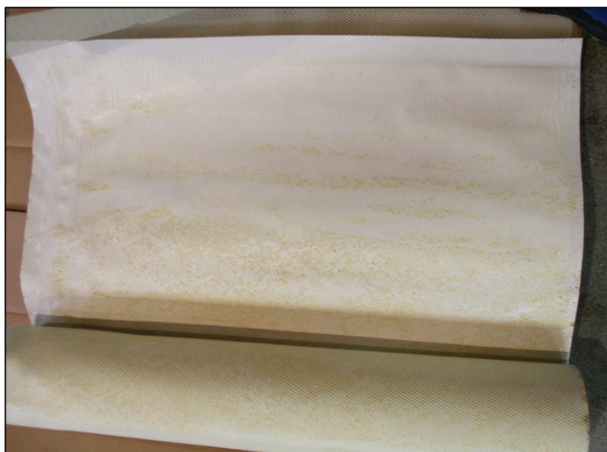
Figure 14 Fouled membrane element from another production facility.
