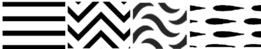
Figure 10. Different PCHE channels: straight, zigzag, S shaped and air foil (from left to right) (Zhang,2016)
