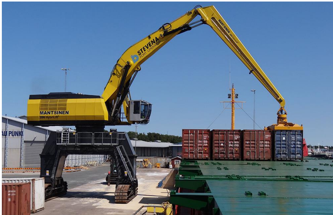
Figure 4.1. Mantsinen 200 with tracks moving shipping containers. (Mantsinen Group Ltd Oy, 2018).
