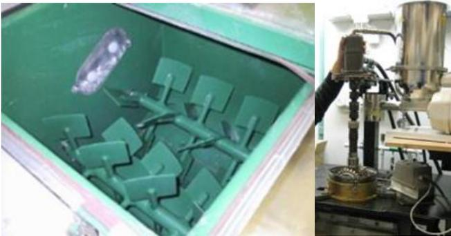
Figure 14: A blade-type blender (right) and the compactor device for fluffy fibre material treatment (left).
