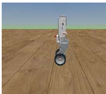
Fig. 7. Virtual model of the Lego Mindstorms self-balancing robot. The model is linked to the Simulink model in a similar way to the TRMS application shown in Fig. 6 c).
