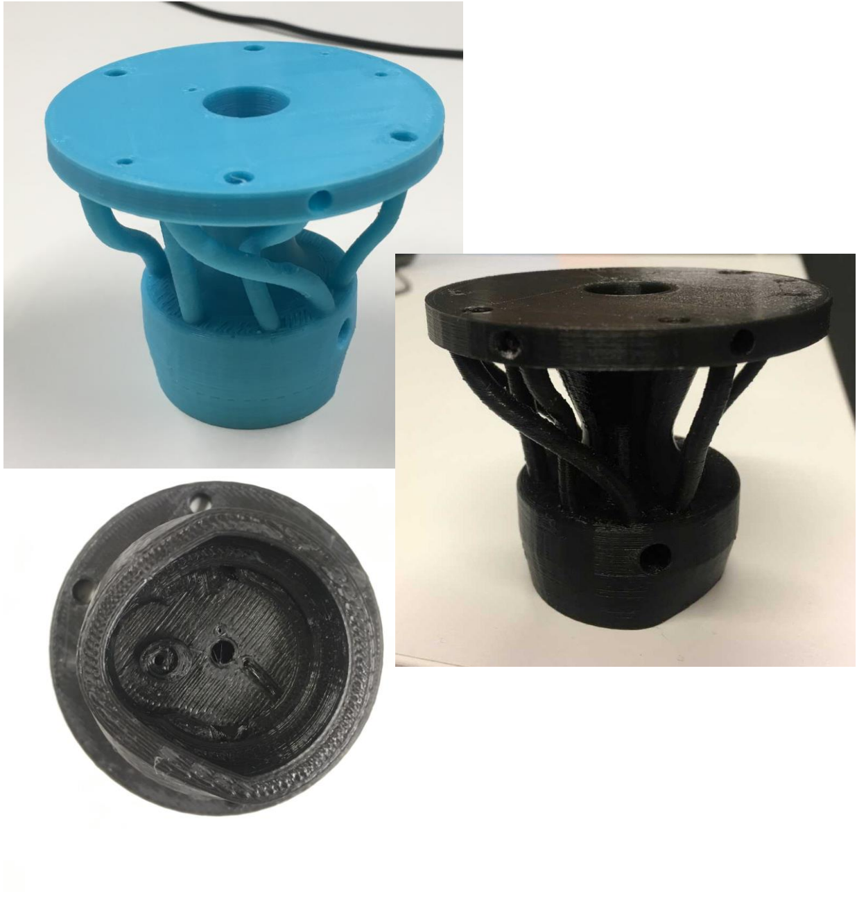
Figure 38: FDM printed final design of the proposed nozzle
