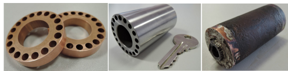
Fig. 10: The rotor elements for brazing assembly and the rotor after brazing
