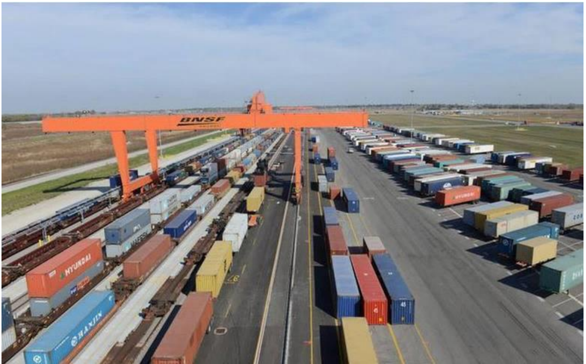
Figure 1. BNSF Railway RMG operating in railway terminal (The Kansas City Star 2015).
