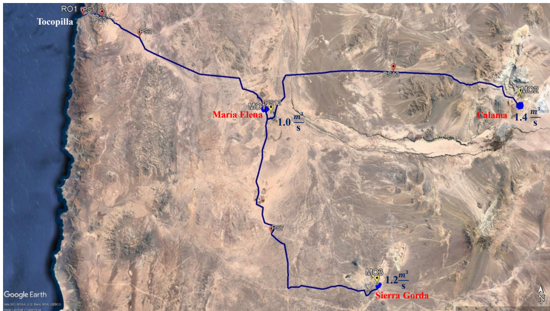
Fig. 7: Integrated water supply system
