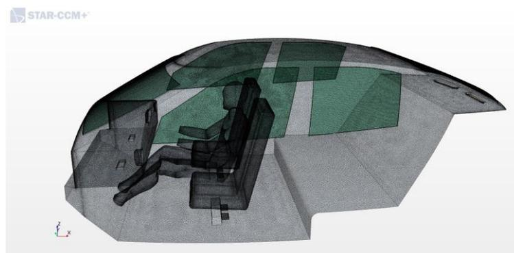
**Figure 33.** Mesh generation in Star-CCM+.
