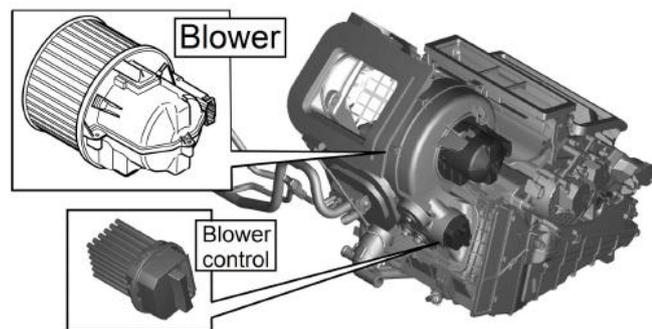
**Figure 7.** Components of HVAC unit. (Nielsen, F. 2016)
