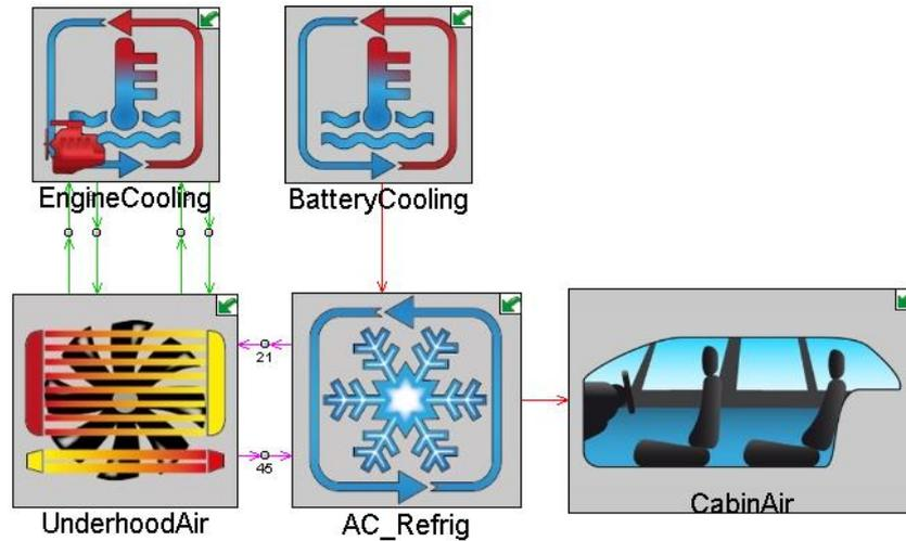
**Figure 18.** Overall 1D model of EV's thermal system in GT-Suite for cooling mode.
