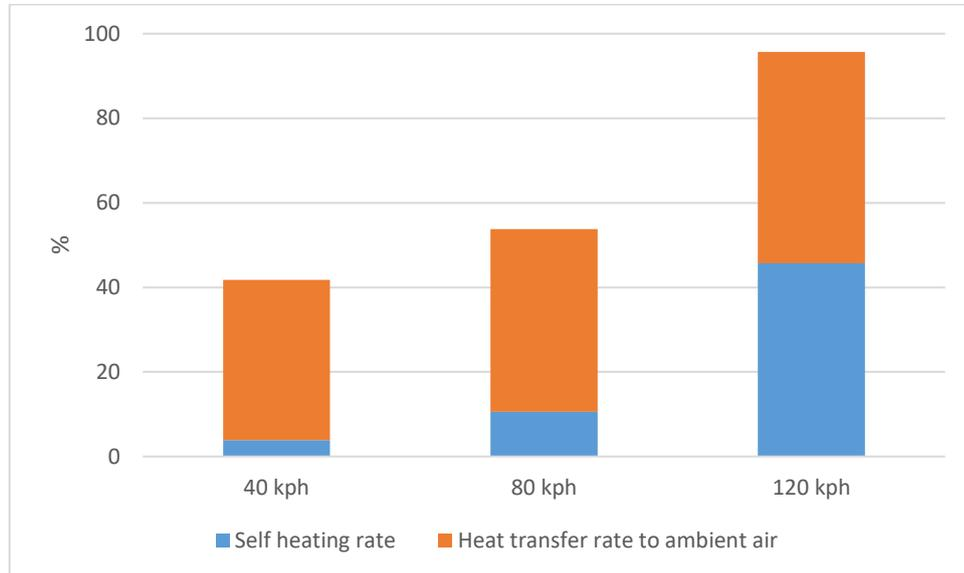
**Figure 27.** Heat loss in RESS box for heating mode.
