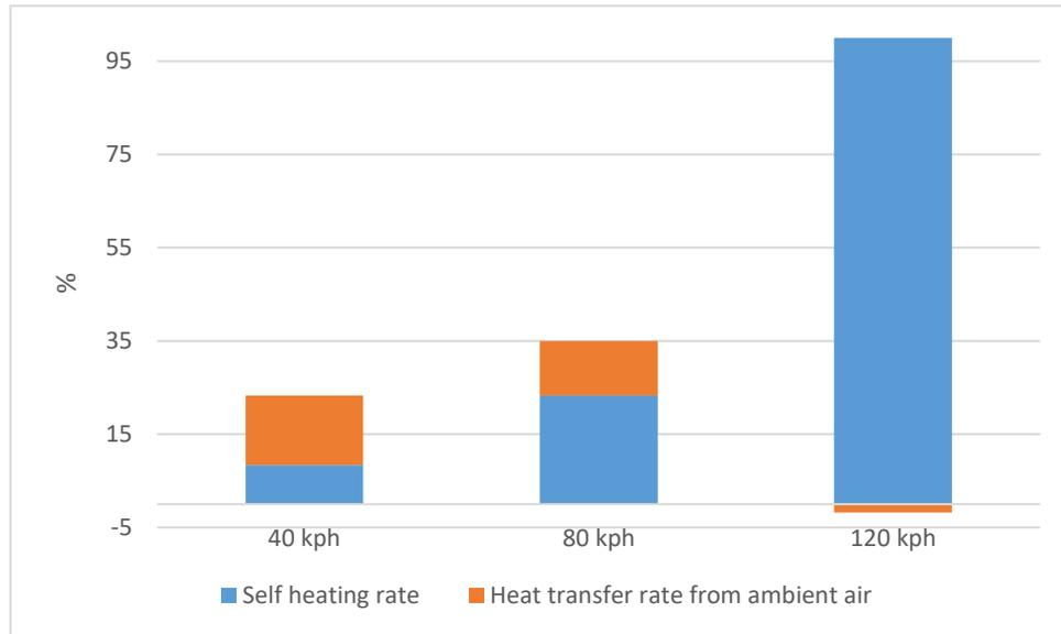
**Figure 22.** Heat loss in RESS box for cooling mode.
