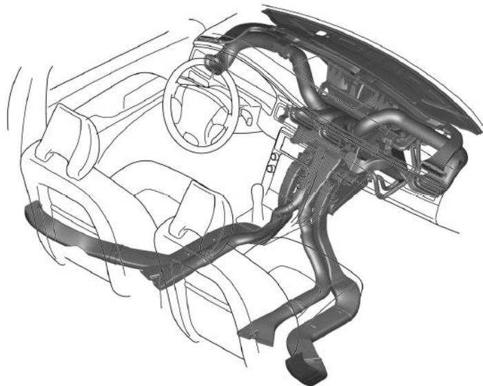
**Figure 11.** Air distribution and ducts of HVAC system. (Nielsen, F. 2016)
