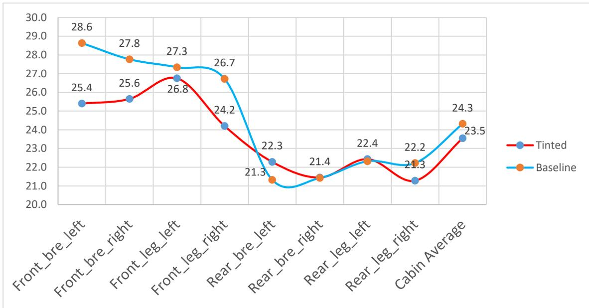
**Figure 40.** Temperature distribution of cabin air volume for cooling mode.
