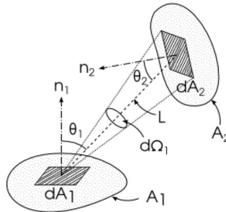
**Figure 14.** Geometry of surfaces. (Lidar, 2018)
