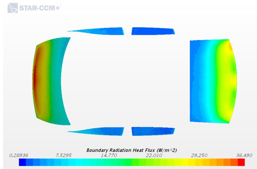
**Figure 37.** Boundary radiation heat flux for baseline scenario.
