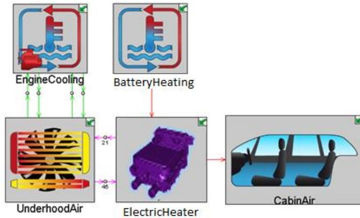
**Figure 19.** Overall 1D model of EV's thermal system in GT-Suite for heating mode.
