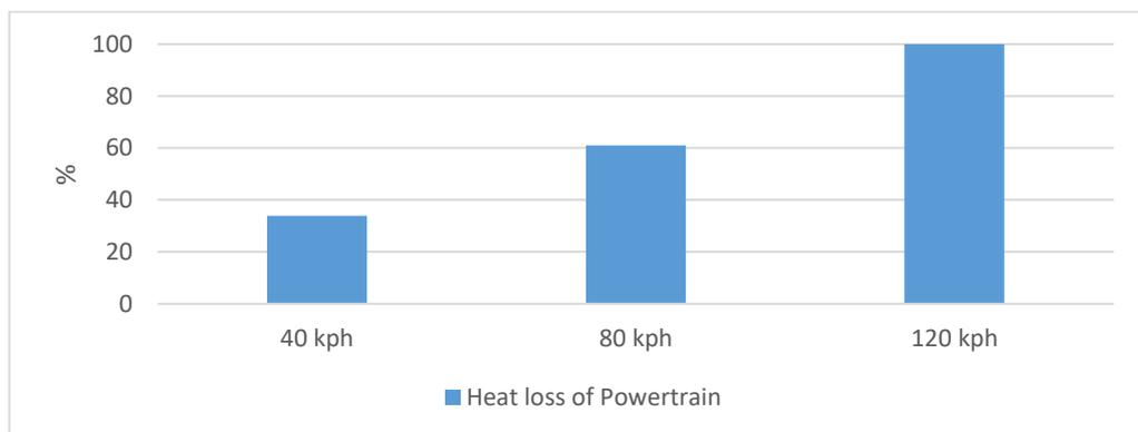
**Figure 23.** Heat loss in propulsion loop for cooling mode.
