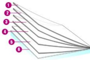
**Figure 43.** Construction of tinting layer. (Solarscreen.eu, 2018)
