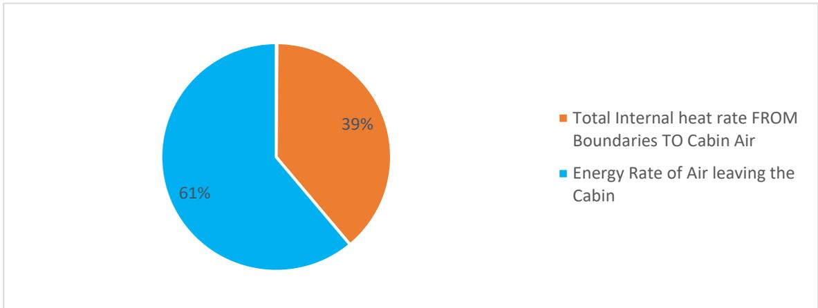
**Figure 25.** Sources of heat loss in EV's cabin for heating mode.
