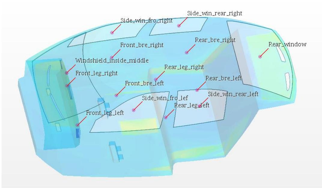
**Figure 39.** Measurement points for temperature distribution inside cabin air volume.
