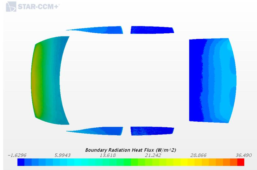
**Figure 38.** Boundary radiation heat flux for tinted glass scenario.
