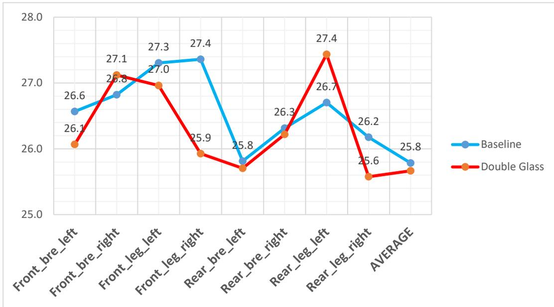
**Figure 42.** Temperature distribution inside the cabin air volume for heating mode.
