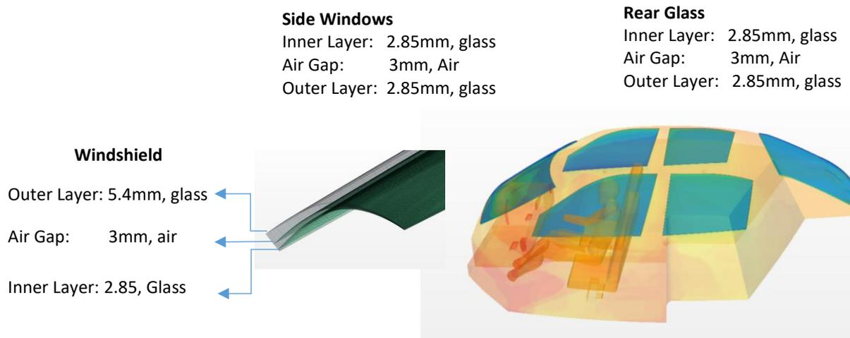
**Figure 36.** Boundary conditions of double-pane glass.
