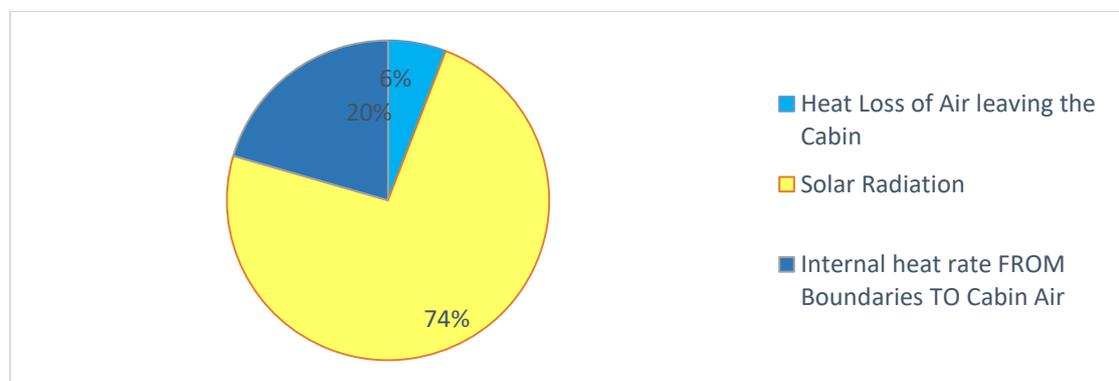
**Figure 20.** Sources of heat gain in EV's cabin for cooling mode.
