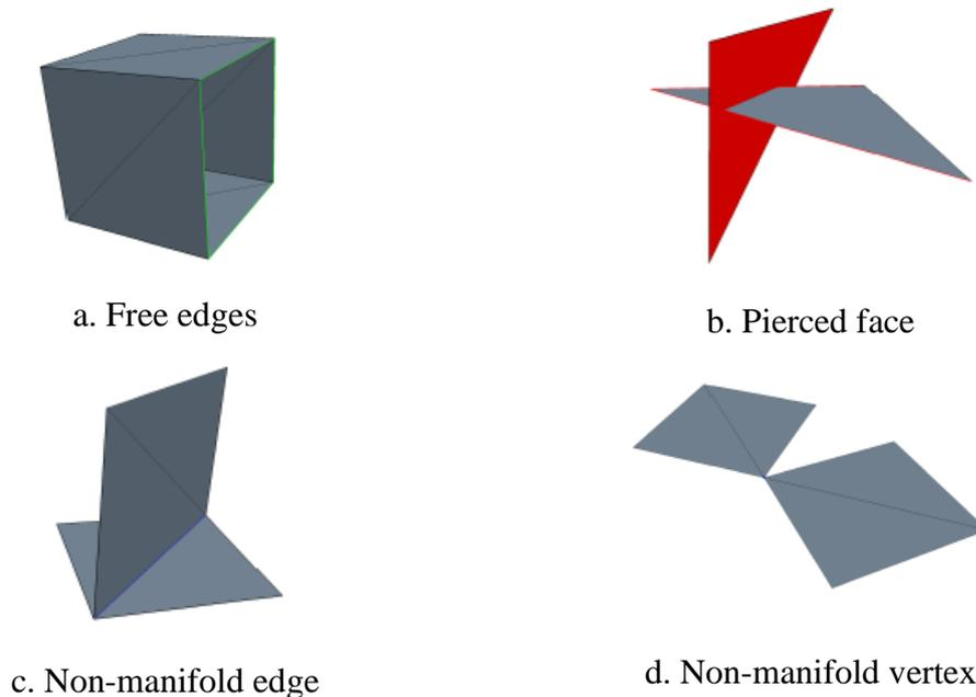
**Figure 31.** Errors in surface preparation in Star-CCM+.
