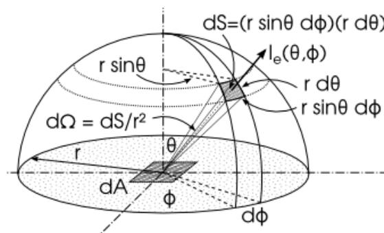
**Figure 13.** Geometries for calculating radiation intensity. (Lidar, 2018)
