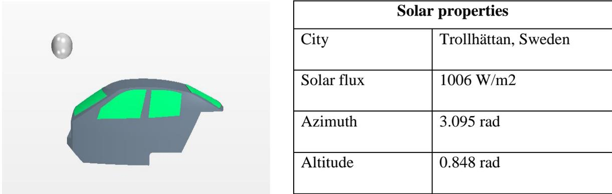
**Figure 34.** Schematic of sun position against vehicle's cabin.
