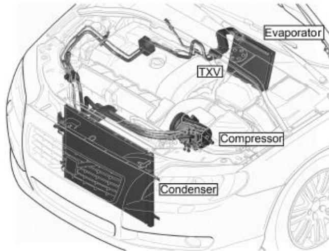
**Figure 8.** Components of AC system. (Nielsen, F. 2016)
