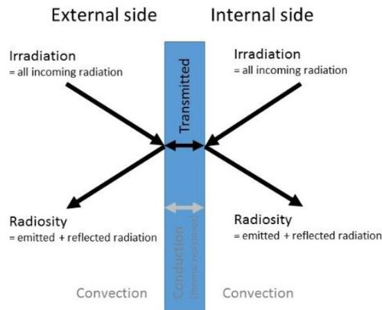
**Figure 30.** The reflection and refraction of solar radiation in vehicle's glass.
