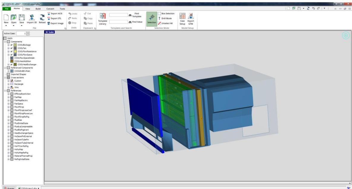
Figure 46. Quasi 3D model of underhood in Cool 3D.
