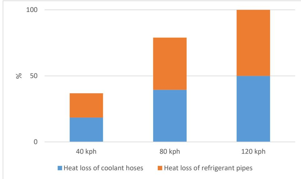
**Figure 24.** Heat loss in pipes and hoses for cooling mode.
