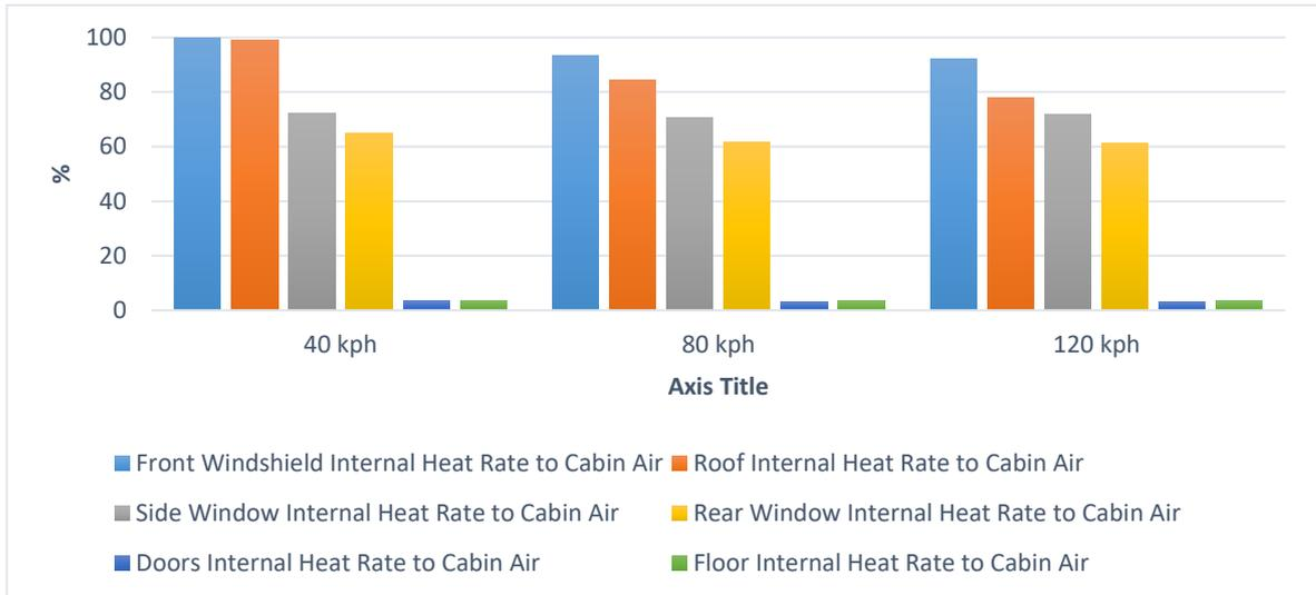
**Figure 21.** Heat gain via different boundaries of EV's cabin in cooling mode.
