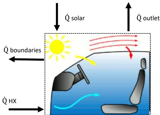
Figure 15. Thermal energy balance inside the cabin.
