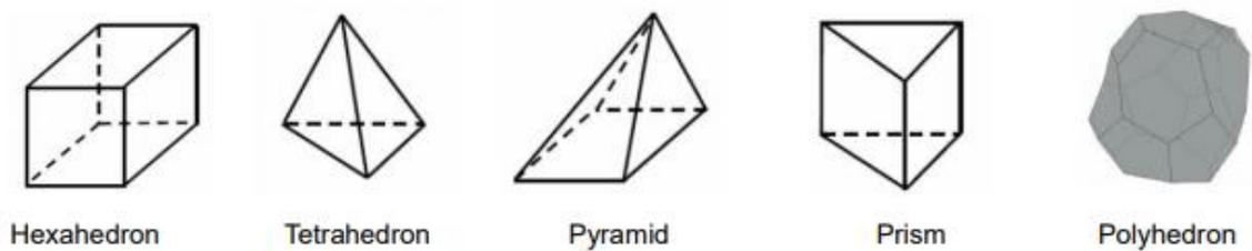
**Figure 32.** Options for structured volume mesh in Star-CCM+.
