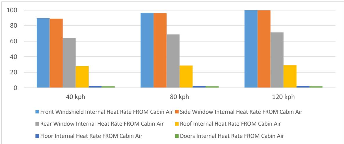
**Figure 26.** Heat loss via different boundaries of EV's cabin in heating mode.
