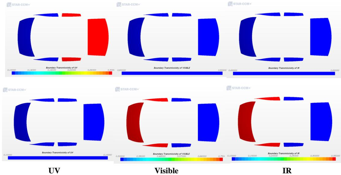
**Figure 35.** Boundary condition of transmissivity for windows for baseline (up) and tinted glass (down).
