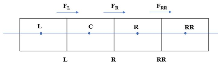
**Figure 17.** One dimensional grid with, center point C, Left point L, Right point R, and Right of Right (RR). Faces L, C and R are between the control volumes and grid flux at each face is  $F_L$ ,  $F_R$ ,  $F_{RR}$ .
