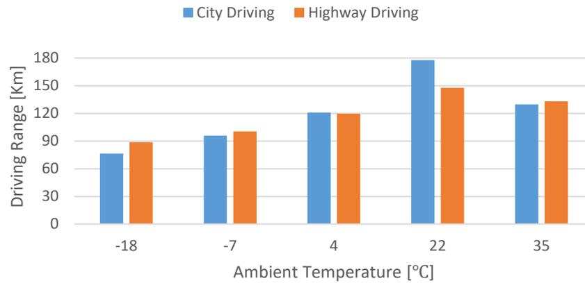
**Figure 1.** Effect of ambient temperature on driving range of Nissan Leaf, HVAC system turns off in 22°C (Stutenberg, 2014).
