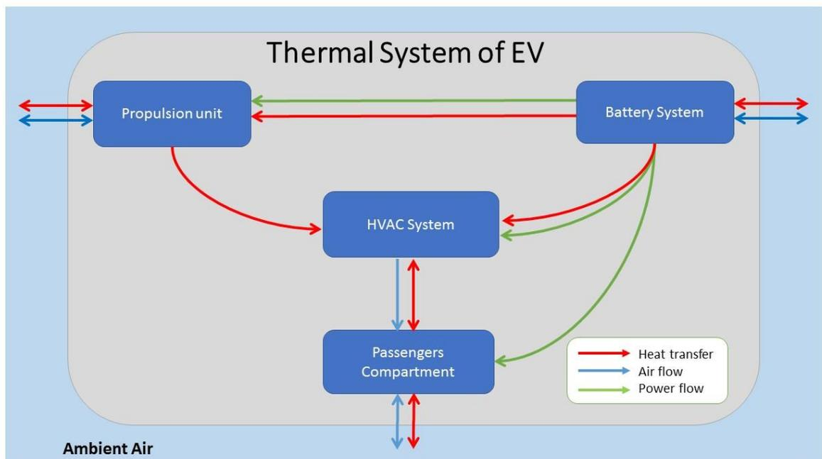
**Figure 3.** Schematic model of Thermal Management System in EV.
