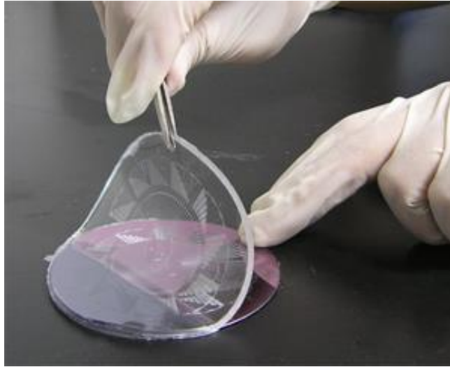
Figure 2.4. Peeling off the cured PDMS slab including the microchannels.[49]
