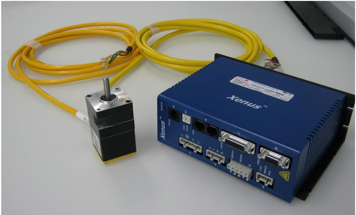
Figure 5.3. Purchased servo motor and the copley control xenus servo drive/controller.
