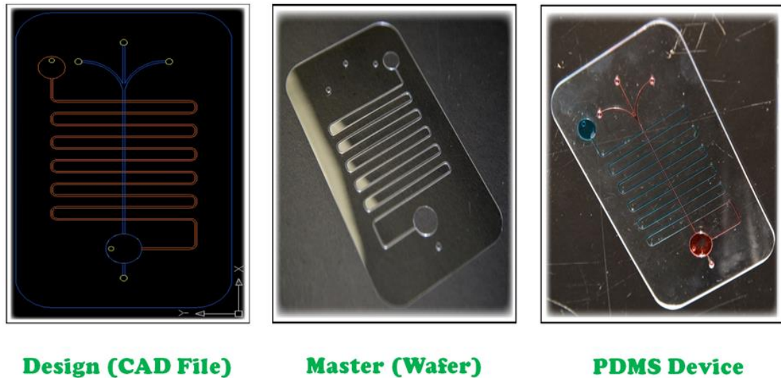
Figure 1.6. Fabrication steps of a PDMS microfluidic device from initial layout to master fabrication and eventually making PDMS device.[60]
