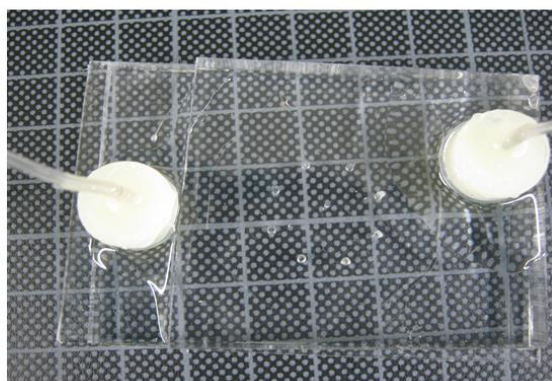
Figure 8.8. Fabricated devices as the result of new protocols for fixing the inlet pins (a) applying uncured PDMS, and (b) applying glue and uncured PDMS over it.
