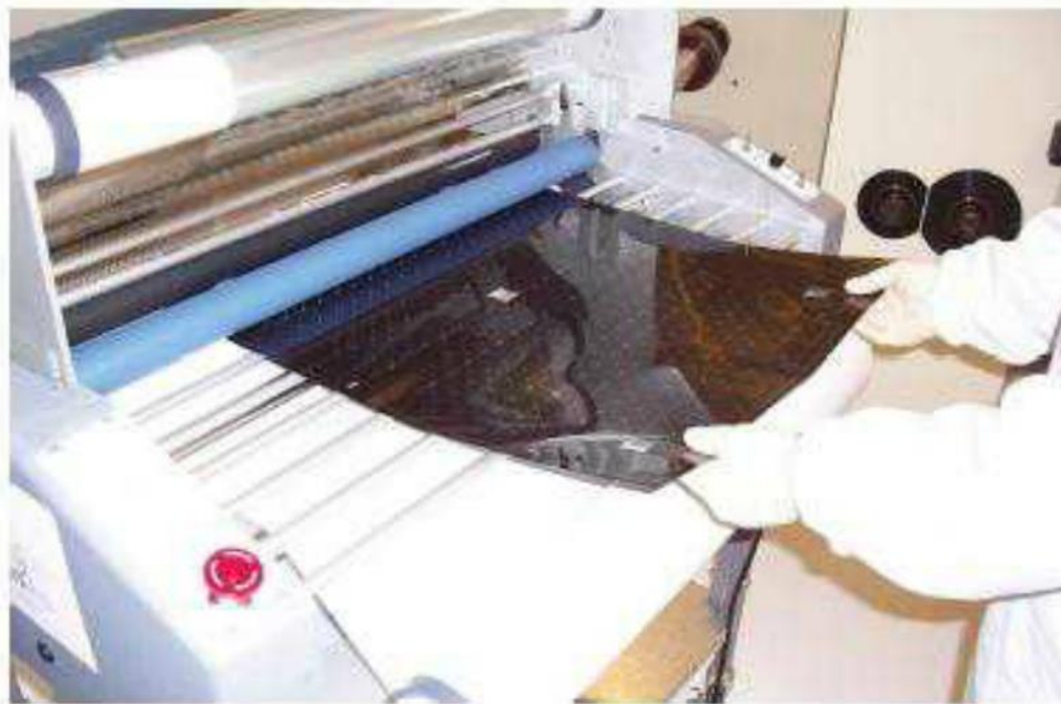
Figure 1.7. A commercial photomask printer while printing a photolithography mask.[71]
