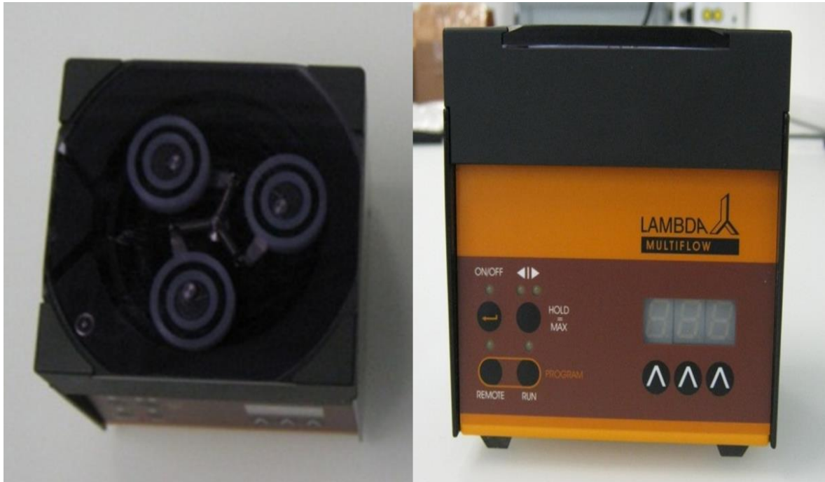
Figure 5.2. Purchased peristaltic pumps from front and up view.
