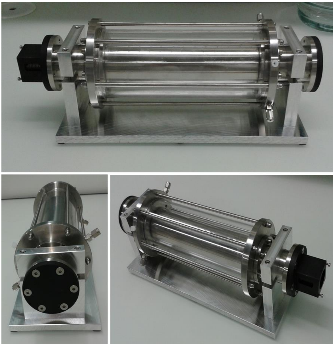
Figure 8.13. The constructed optimized Taylor-Couette device for droplet generation.
