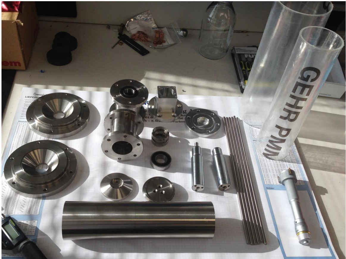
Figure 8.12. The parts of Taylor-Couette device ready for assembling.
