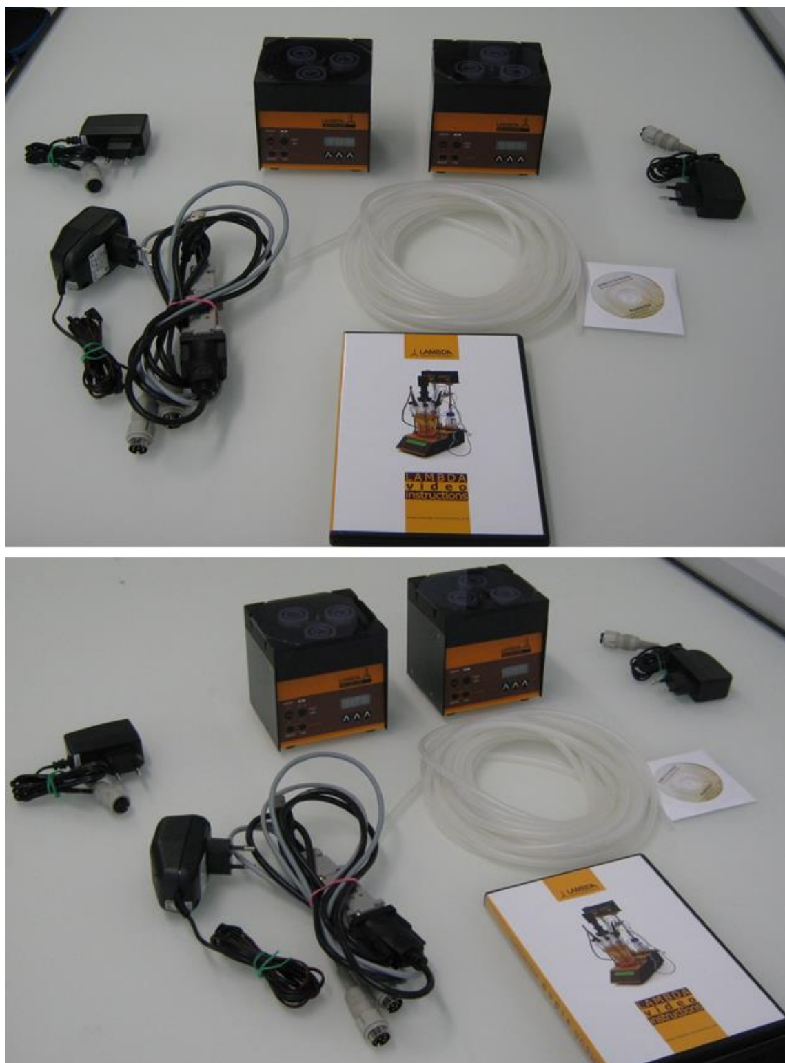
Figure 8.10. Two purchased identical peristaltic pumps and their accessories.
