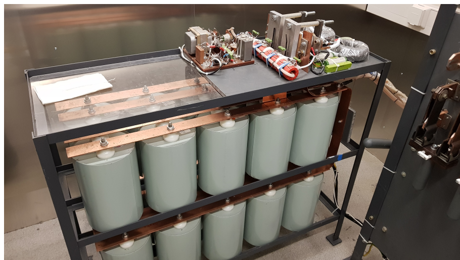
Figure 8. The capacitor bank. The thyristor discharge circuit (as depicted in Figure 7) can be seen on top.
