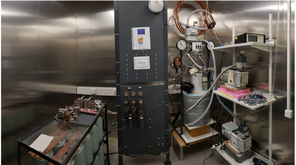
Figure 3. The apparatus in the measurement room. Note the magnetic shielding on the walls.
