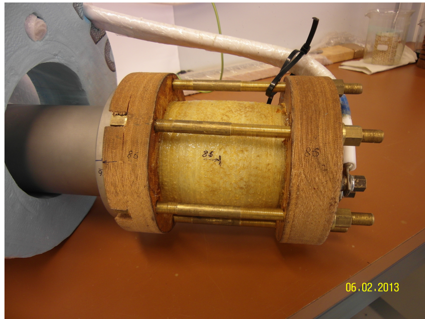
Figure 4. The pulse solenoid attached to the end of the internal cryostat.
