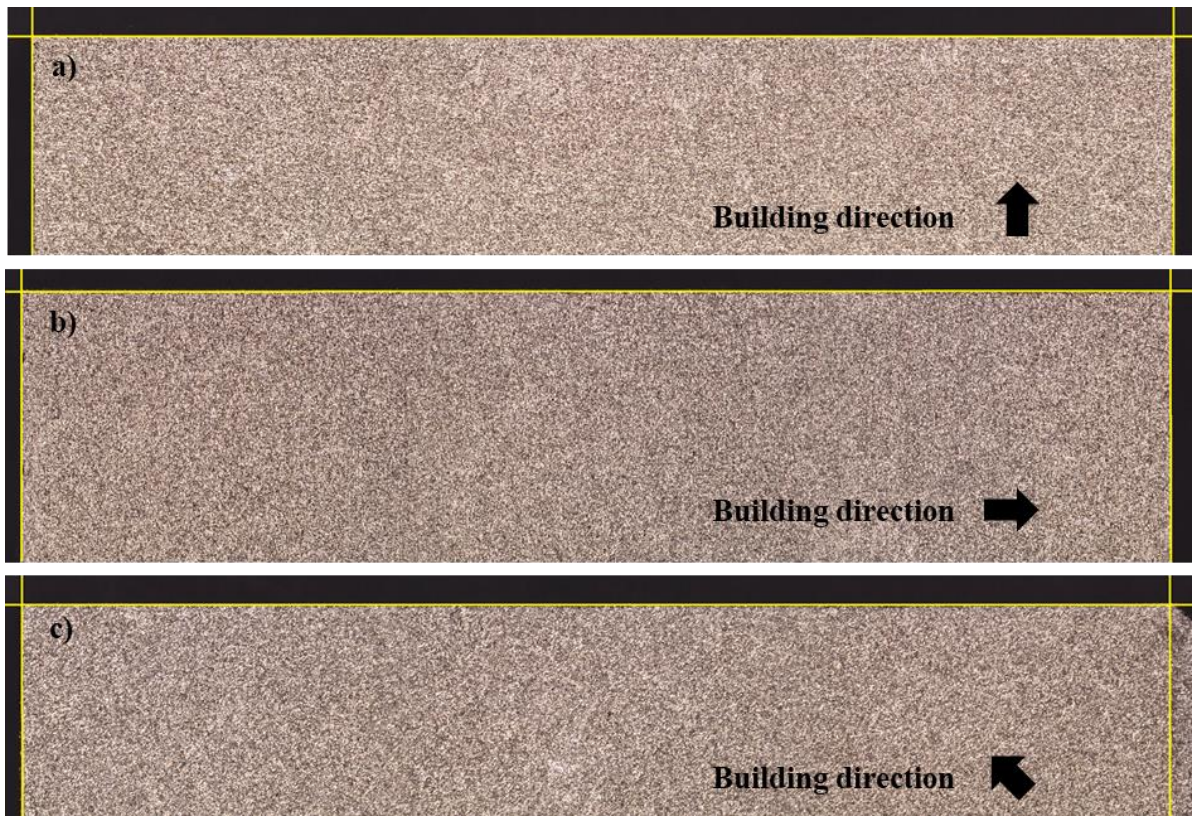
Figure 49. Macrographs of test samples (a) D1, (b) D2 and (c) D3 (support structures removed from bottom surface). Front view, building direction is indicated with arrow.
