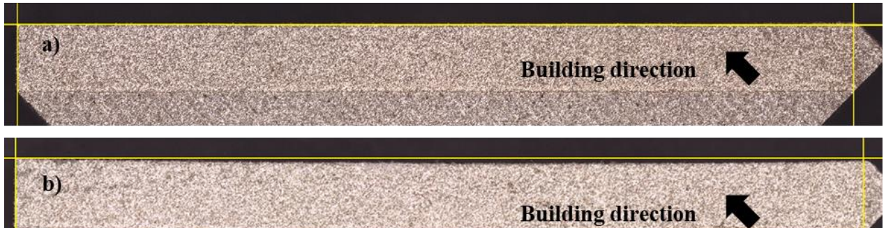
Figure 47. Macrographs of test sample C4 (a) with support structures and (b) without support structures. Front view, building direction is indicated with arrow.
