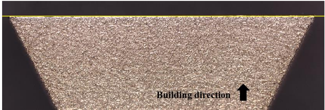
Figure 54. Macrograph of test sample E2. Front view, building direction is indicated with arrow.
